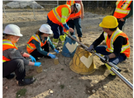
NWMO staff and industry experts collect deep water samples for microbiological analysis.
