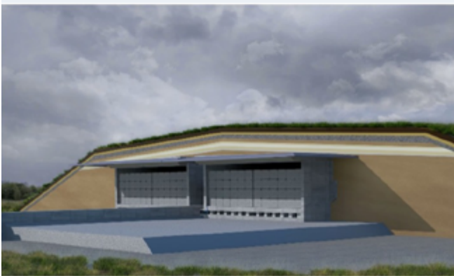
Graphic representation of a cross-section through the filled, structurally enclosed and covered surface disposal facility.
