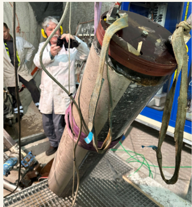
CIM "active" overcore showing the contact between cement and granodiorite.
