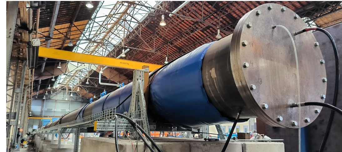
Full-scale mockup of the carbon steel lining designed to test inerting processes
