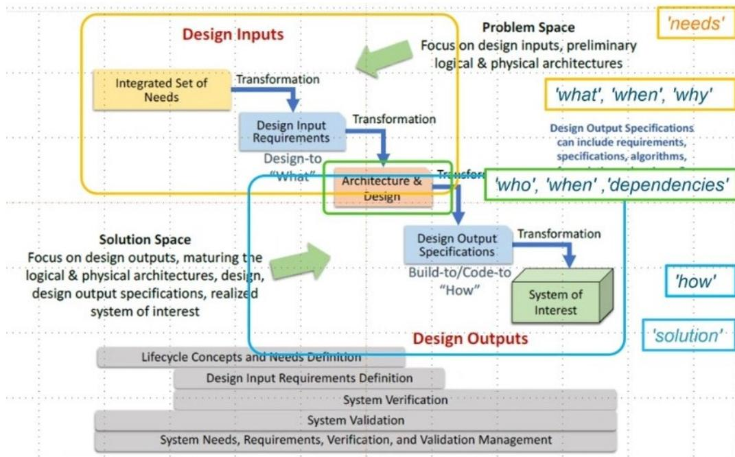
Figure 3 – Requirements Management System: design and implementation process [16]
