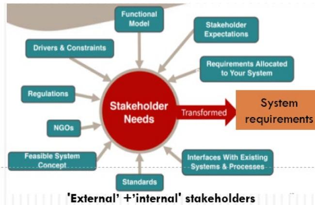
Figure 6 – Transforming stakeholder needs into requirements [1]
