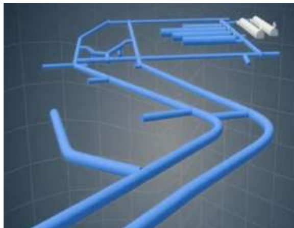
Figure 82 – Facility has six chambers for storage of containerised low- and medium-level radioactive waste [115]
