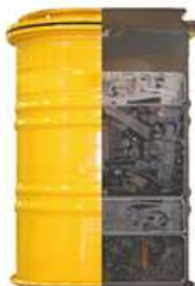
Figure 18 – Not radioactive sample of NES standard waste drum with pellets
