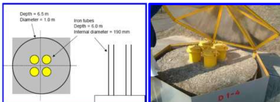
Figure 55 – Shallow boreholes for DSRS in Hungary [93].
