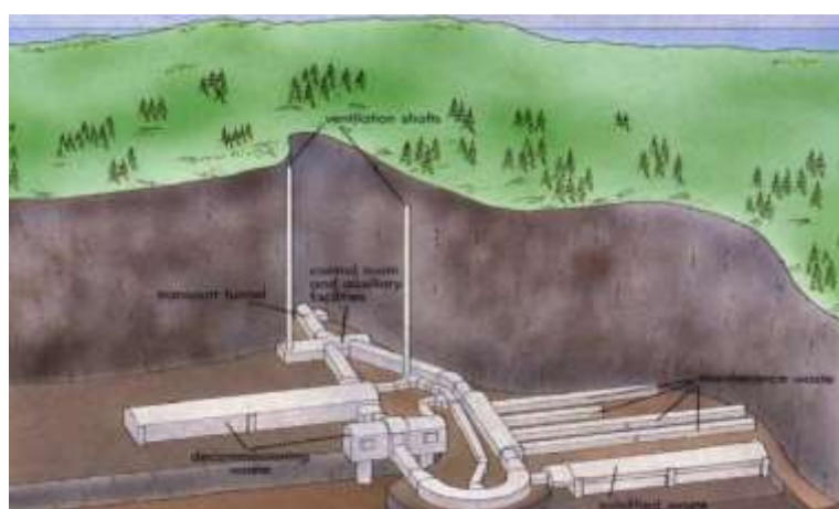
Figure 85 – Loviisa disposal facility layout [123]
