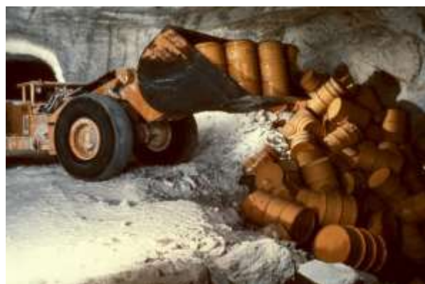
Figure 75 – Dumping of drums (LLW) with a wheel loader (since 1971) [116]
