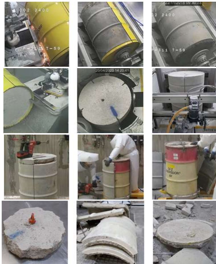
Figure 28 – Reconditioning of inhomogeneously cemented drum
