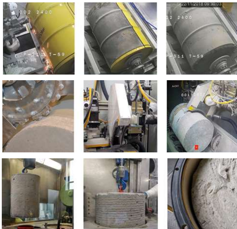
Figure 26 – Reconditioning of homogeneously cemented drum
