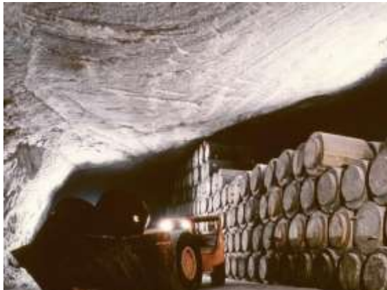
Figure 72 – Horizontal storage of drums (LLW) with a lost concrete shielding (1978) [116]
