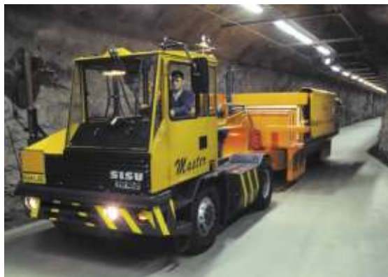
Figure 86 – Low- and intermediate-level waste is transported to the final disposal facility in a specially designed vehicle. The vehicle and the load are checked before they are taken into the disposal facility. The unloading is carried out by remote controlled crane [95]
