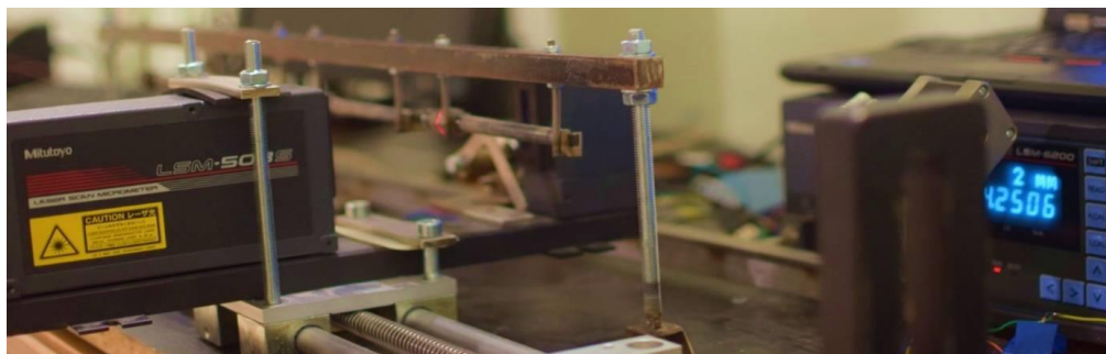
Figure 43 – Laser profilometry setup with measuring head of the laser micrometer mounted on the linear module (left), micrometer control unit and data acquisition laptop (right), and the cladding sample on the sample holder (middle)
