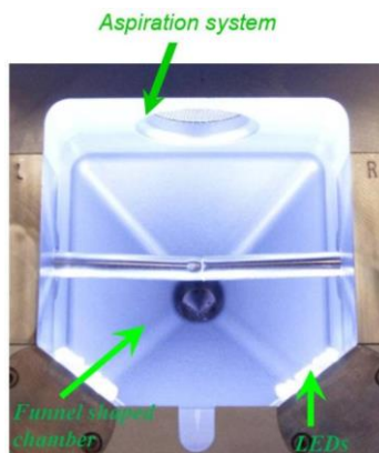
Figure 6 – Inside view of the closed test chamber of the impact device after a dummy cold test (cladding tube filled with aluminium pellets)
