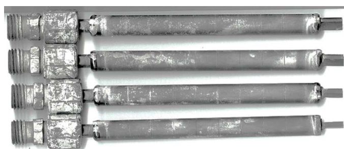
Figure 48 – Picture of the four measured samples with the hydraulic connectors attached at the end of the first test series
