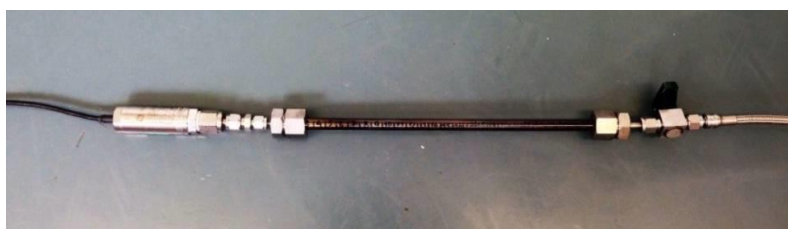
Figure 9 – Gas-tight sample assembly connected to a pressure gauge and fitted with a pressure transducer, ready for mechanical testing
