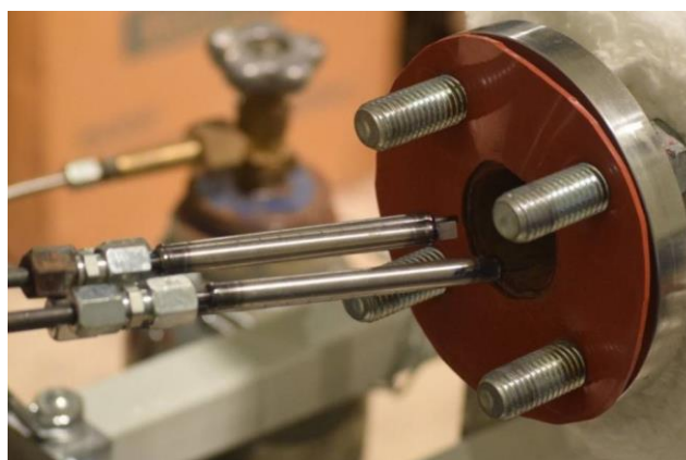
Figure 45 – Samples connected to the pressurisation system entering the tube furnace
