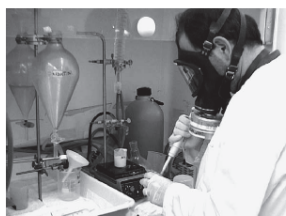
Fig.3. Addition of Pb(NO 3 ) 2 to the iodide solution to precipitate lead iodide.
