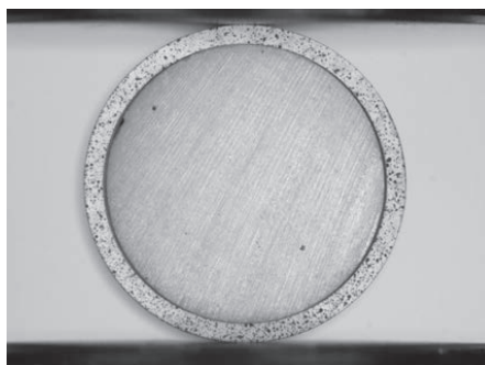
Image of sample with insert and circumferential hydrides during RCT at same load
