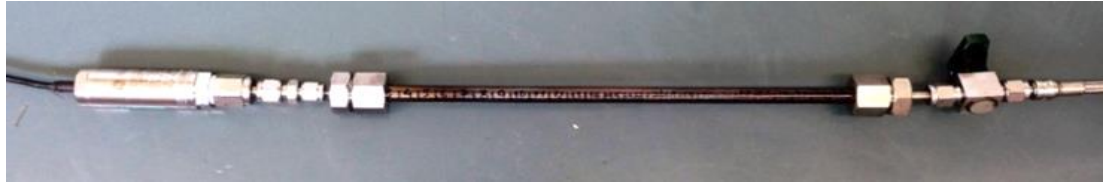
Figure 22 – Gastight specimen assembly connected to the pressure gauge with attached pressure transducer, ready for mechanical testing
