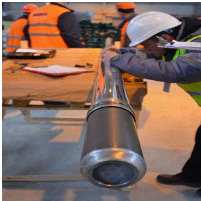
Figure 14 – Fuel tube in which FR bundles will be stored
