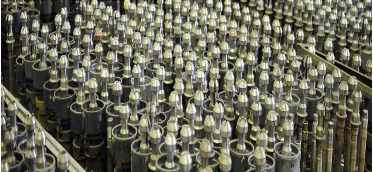
Figure 10 – Storage of RBMK-1000 SFAs in ISF-1 “wet” storage facility
