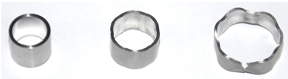
Figure 4-8: Deformations caused by the mandrel tool. On the left is an 8 mm as-received E110opt ring, in the middle after 30% diameter increase and on the right side, a torn sample with an inner diameter increased by about 80%.
