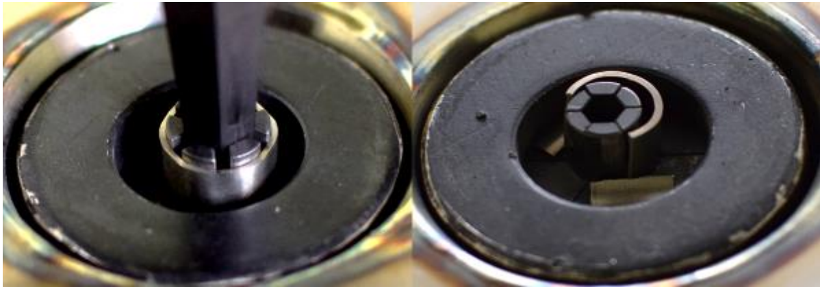
Figure 4-9: Mandrel tests of hydrogenated E110opt samples at room temperature after 15% inner diameter increase. The left sample (PHG-53, 489 wppm hydrogen) still exhibited ductile behaviour while the right sample (PHG-83, 2059 wppm hydrogen) was brittle and broke.
