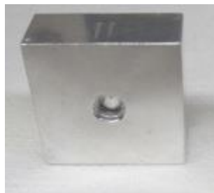
Figure 2-2: Custom built sample holder for XAS measurements of fuel fragments and cladding segments.
