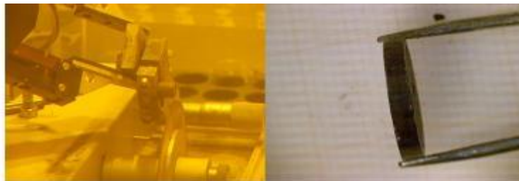
Figure 2-1: Cutting process of a 2 mm thick disk of the MOX fuel specimen.
