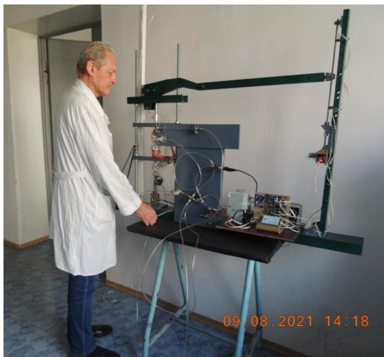
Figure 8.2 – KIPT laboratory installation to measure the permeability and swelling pressure of PBC bentonite at a temperature > 100°C
