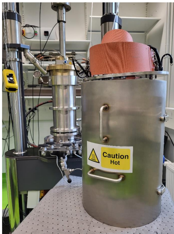
Figure 9.3 - Triaxial cell temperature control system with heating elements, insulating covers and a heater pack.
