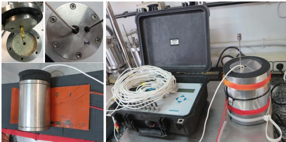
Figure 4.1 – Cell assemblage: hole drilled on the bentonite surface to insert the sensor, sealing of the cable inlet with thermoresistant silicone, wrapping with heating mat and insulating material (left); cell in operation with a psychrometer inserted
