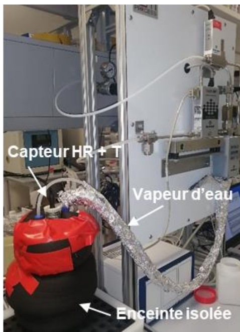
Figure 3.2: Used device for isotherm determination. Capteur is the sensors for humidity and temperature . Vapeur shows the water vapour. Enceinte isolée is an isolated enclosure. Poudre is the clay powder and cellules is reaction cells.
