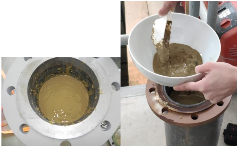
Figure 6.2 Wet bentonite before treatment poured into the vessel (left). Sampling of wet bentonite after 6 months of thermal treatment (right)
