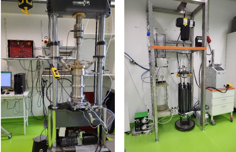
Figure 11.1 The triaxial device (left) and the self-built alternative experimental system for isotropic compaction (right).
