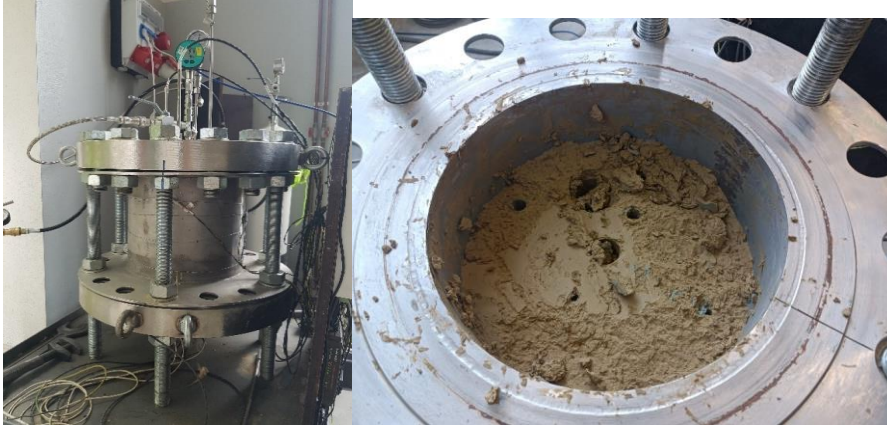
Figure 6.3 Medium-scale experiment (left) and bentonite inside the experiment during dismantling (right)
