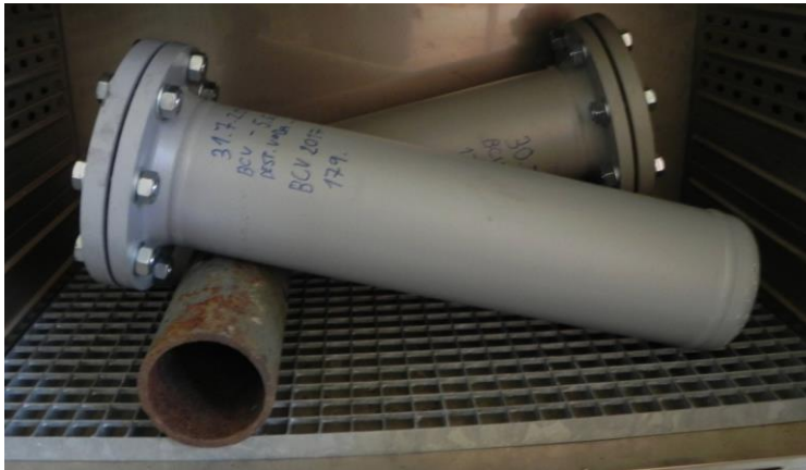
Figure 6.1 Pressure vessel for thermal treatment of wet bentonite
