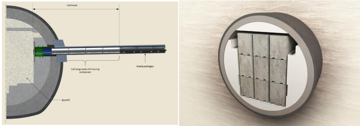
Figure 2-2 Schematic diagram of an HLW cell and arrangement of waste packages in an ILW-LL cell
