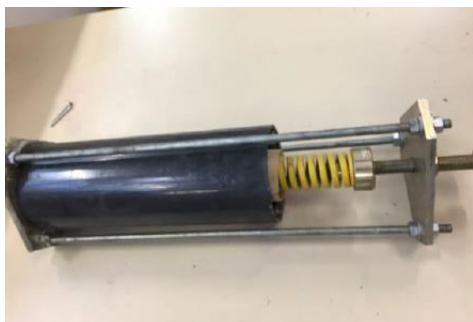
Figure 4-95. Clay preservation packages. As soon as a clay core is brought to surface, it is sealed and confined in these cells in order to try and keep the clay properties as close as possible to its virgin state
