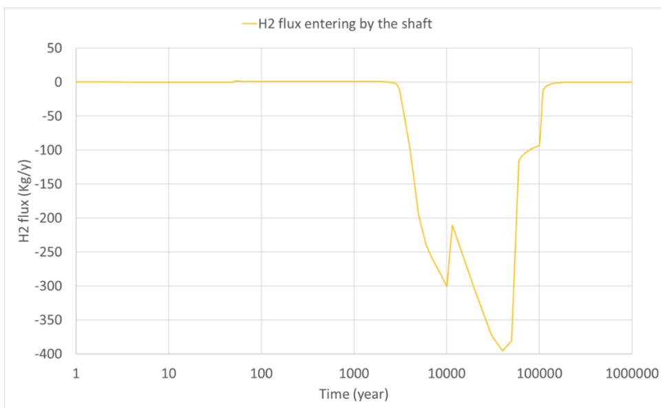
Figure 3-23: Gas flux entering the shaft toward the upper aquifer
