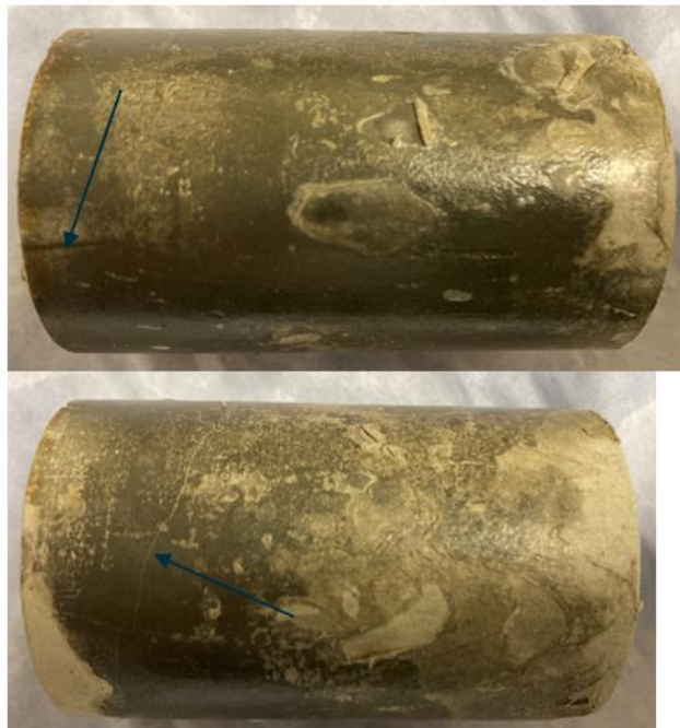
Figure 2.34: Photos of the sample (COx1) after removal from the apparatus with small fractures highlighted.
