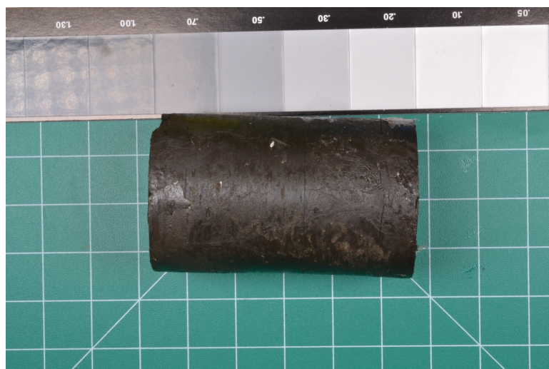
Figure 2.55: Photo of sample BC2 after removal from the apparatus with small fractures seen parallel with bedding.
