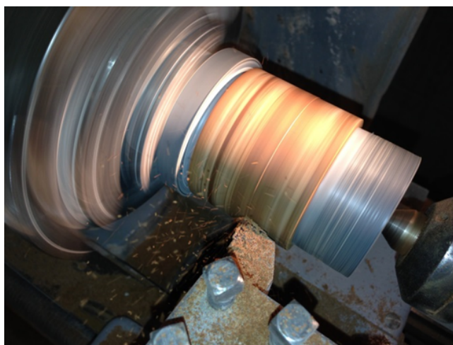
Figure 2.26: Callovo-Oxfordian Claystone sample being cut on a lathe during the careful sample preparation process.
