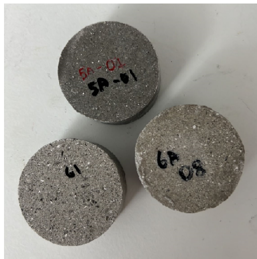
Figure 1.36: plugs of synthetic clay samples for diffusion tests. (Legend: 5A-01 – composition 5A, 6A08- composition 6A, 61- composition 7.)
