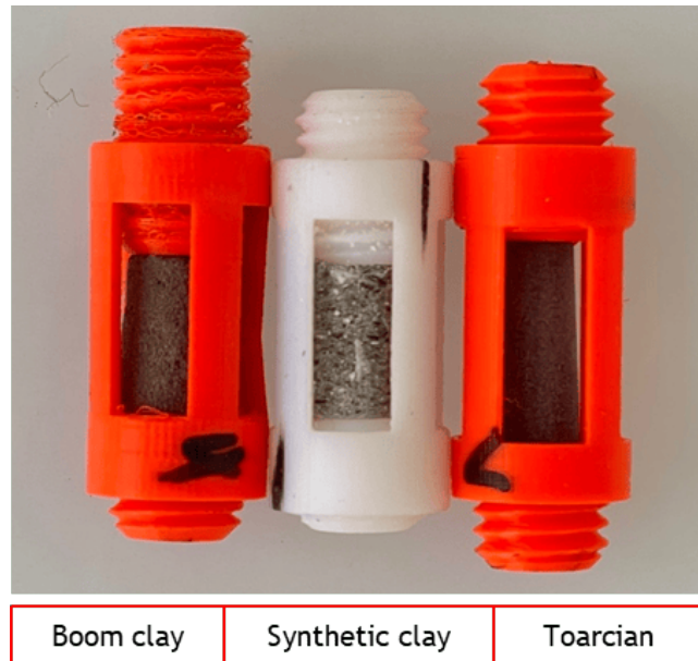
Figure 1.81: Specimens of the three clays in containment cells
