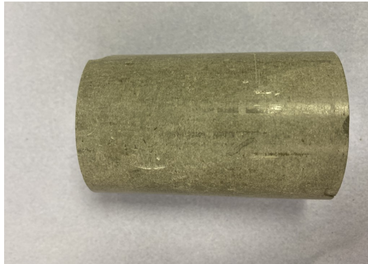
Figure 2.28: Sample of Callovo-Oxfordian claystone prepared by machine lathing.
