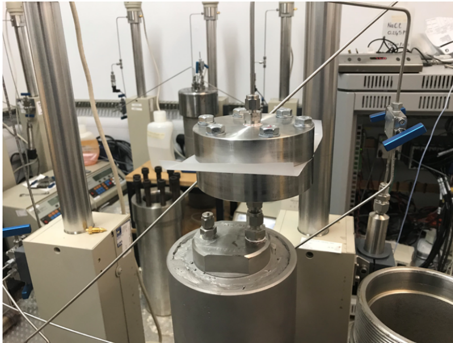
Figure 1.15: Photo of the membrane holder used to estimate the diffusion coefficients of different sheathing materials. Values obtained are conservative, representing upper leakage values.
