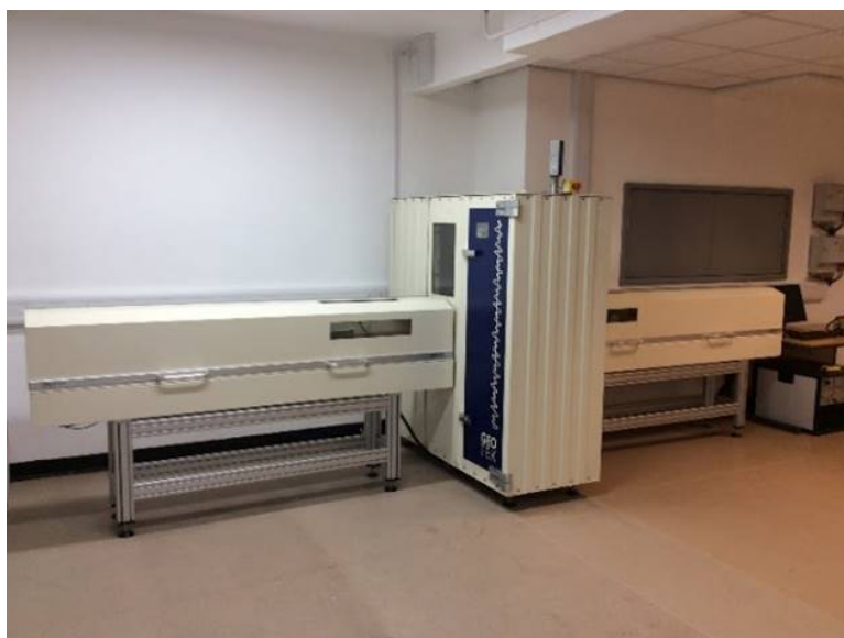
Figure 1.12: Geotek Rotating X-Ray CT scanner in the BGS Core Scanning Facility. The scanner is capable of scanning in both 2 and 3D. For the current study both modes were used. For the three-dimensional image, files were taken in an XY orientation down the length of the sample.
