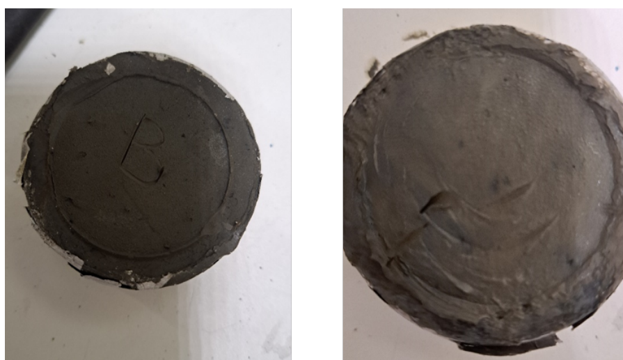
Figure 2.5: Post-test images of the sample, showing no major heterogeneities at the sample surface (left = bottom, right = top of the sample)
