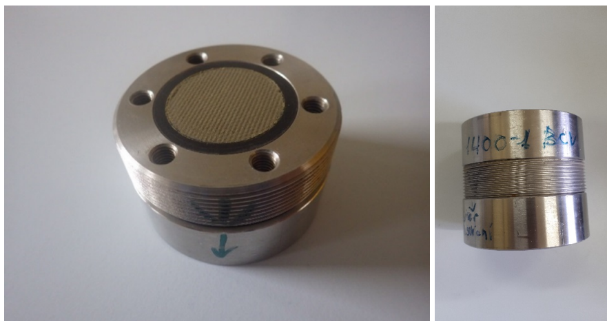
Figure 2.215: BCV bentonite sample inside the stainless-steel cell
