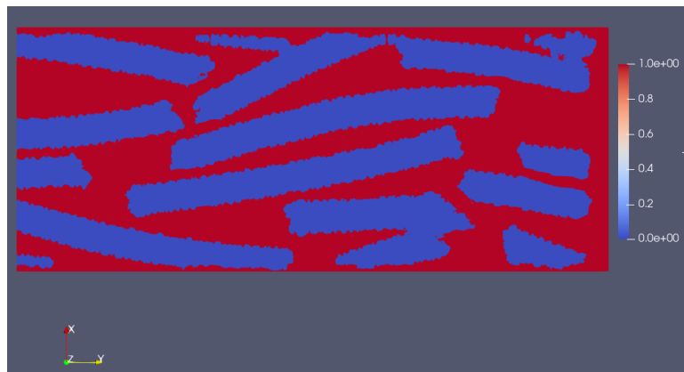
Figure 1.134: Configuration of the 2D clay structure for lattice Boltzmann modeling. Clay particles and pore space are represented by blue and red regions, respectively.
