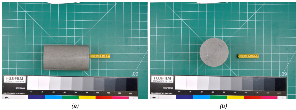
Figure 2.35: Sample of Callovo-Oxfordian claystone prepared by machine lathing.
