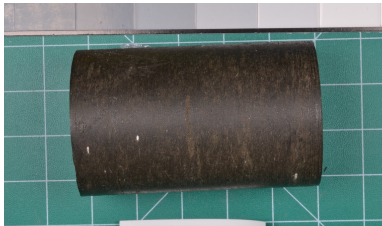
Figure 2.49: Sample of Boom Clay prepared by machine lathing for test BC2.
