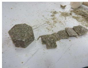
Splitting the core in two, removing external parts, smoothing surfaces
