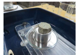
Immersion of the samples in mercury to determine its volume before drying in the oven
