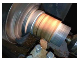
Sample manufacture by machine lathing
