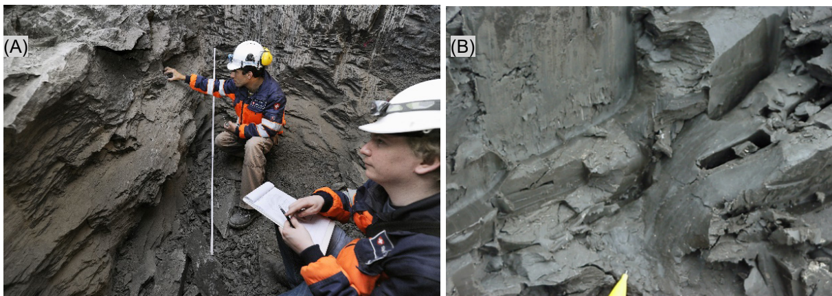
Figure 3-6 – Different types of clayey rocks. (A) Opalinus clay, survey during excavation of a gallery/drift for the Full-Scale Emplacement Experiment (Mont Terri URL, Switzerland) (courtesy of Nagra, @ Comet GmbH Weisslingen, CH). (B) Boom Clay (Belgium) (source: EURIDICE).
