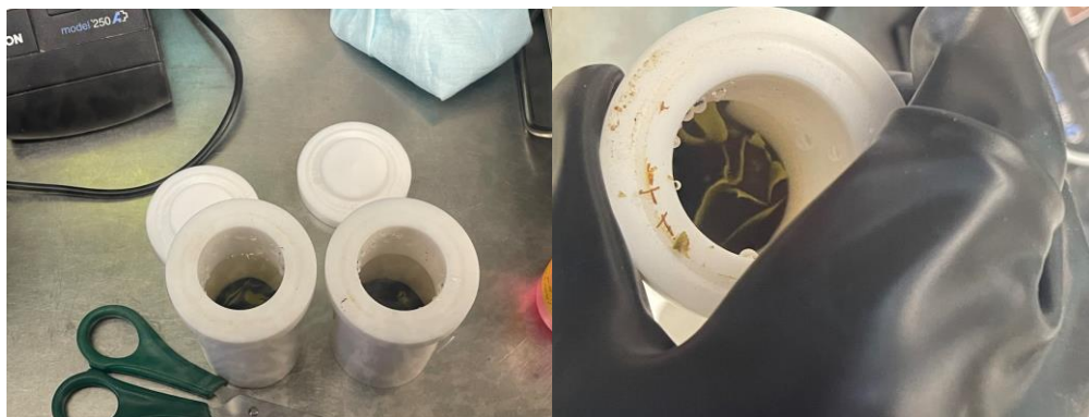
Figure 9. Ferrous smectites at 150 °C and starting pH of 12 synthesized during; a) 4 days; and b) during 30 days.
