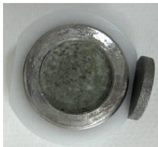
Figure 76. Experimental cell designed to carry out radionuclide in-diffusion experiments in compacted smectite samples mixed with known proportions of different Fe oxides and phases.
