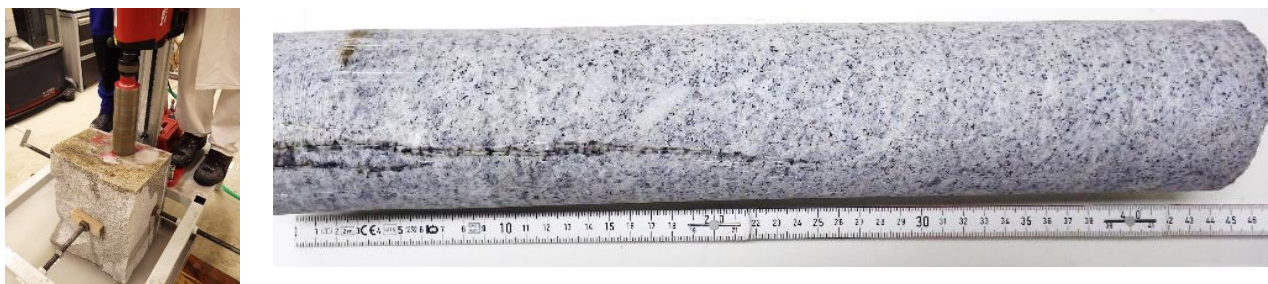
Figure 5-1: Drill core sampling in the preparation laboratory of the UJV from a granite block from the Mrakotin quarry.
