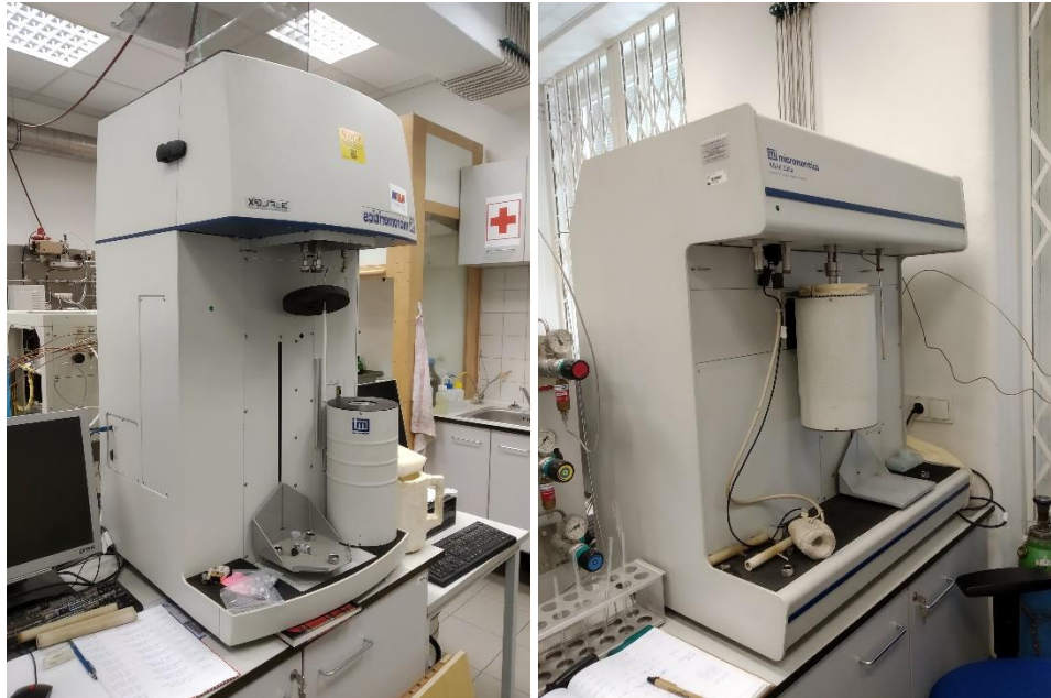
Figure 1-18 Micromeritics 3Flex (left) and ASAP 2020 (right) adsorption analyzers: advanced instruments for adsorption analysis at UCT Prague (Doc. Ing. M. Lhotka, Ph.D.)
