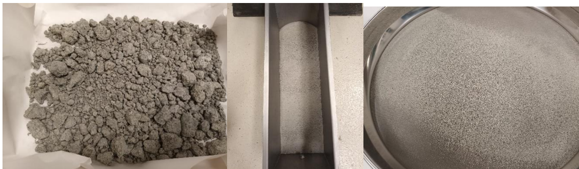
Figure 1-12 Processing stages of the clay infill (from left: drying, crushing and sieving)
