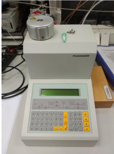
Figure 1-27 "Pycnomatic" helium pycnometer at the UCT Prague (Doc. Ing. M. Lhotka, Ph.D.)
