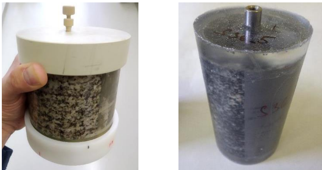
Figure 5-7: Sample MSVJ2 conventionally prepared for migration experiments, sample S36-5 prepared according to the alternative method that minimises the dead volume (right).
