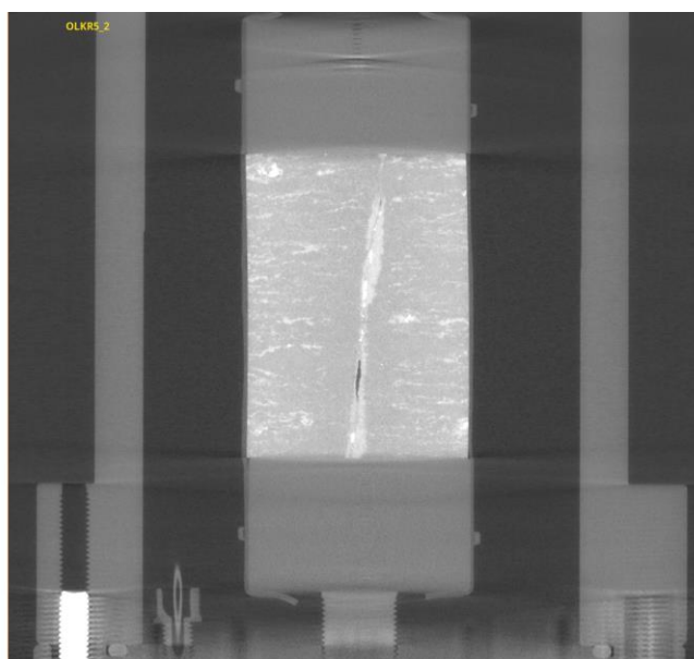
Figure 5-33: Merged high-resolution \mu CT images with a voxel size of 16 \mu m of the entire drill core (ONKALO; sample OLKR5). Dense material is shown in black, grey zones are fracture fill (chlorite and calcite), white is open volume of fracture. Inset: Enlarged section showing the complex structure of the fracture and the position of the different fracture mineralisation.
