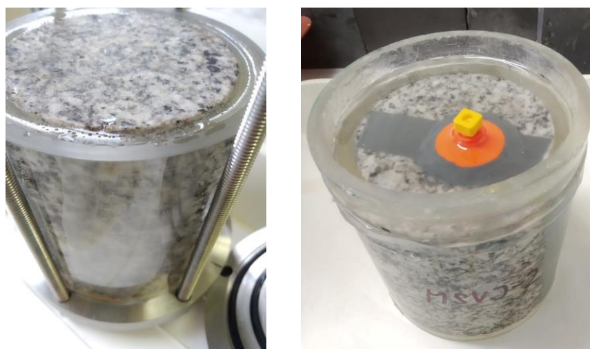
Figure 5-9: Fixing procedure after the leakage of the sample MSVJ2 was detected
