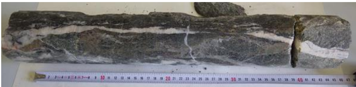
Figure 1-5 Sample of a fracture filling extracted from sampling point BZJXII (38.8 m)
