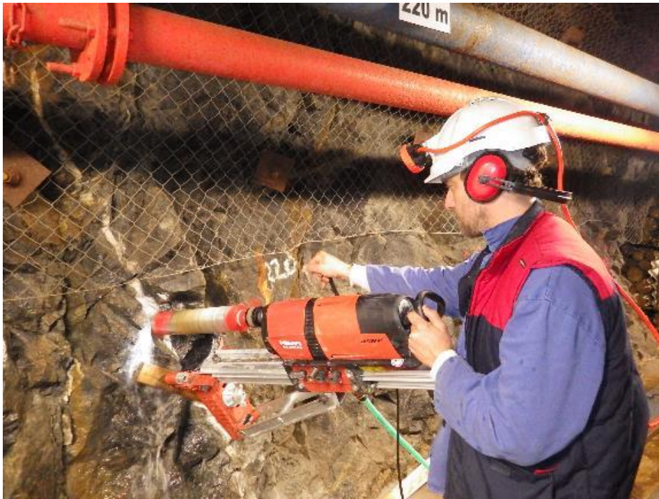
Figure 1-3 Extraction of a sample of a calcite filling in the Bukov URF (sampling point BZJXIJ 219.4 m)
