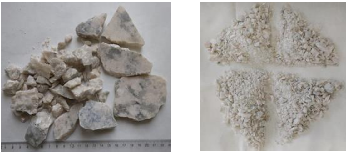
Figure 1-8 Separated calcite material (left) and the quartering of the crushed material for distribution among the research partners (right)
