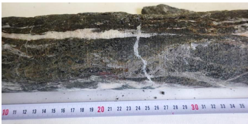
Figure 5-3: Drill core sample BZ8_1 from Bukov URF (BZXII-38,8 m), showing multiple generations of fracture-filling calcite precipitates
