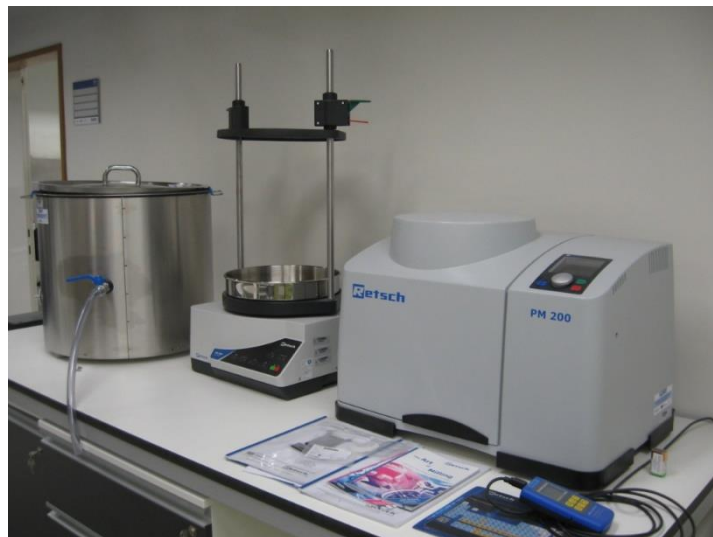
Figure 1-14 Planetary Ball Mill PM 200 (Retsch), Sieving Machine AS 300 (Retsch), and UV Bath for Cleaning Sieves (description of the image from right to left)
