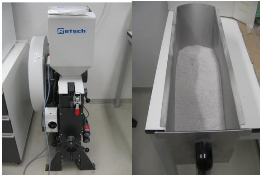
Figure 1-13 On the left: Jaw crusher BB 200 (Retsch), on the right: Crushed rock sample
