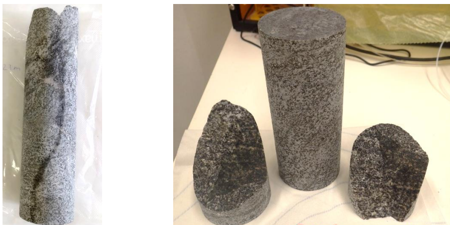
Figure 5-5: The drill core from borehole S36 (Bukov URF, ZK-2), on the left before and on the right after the cutting process.
