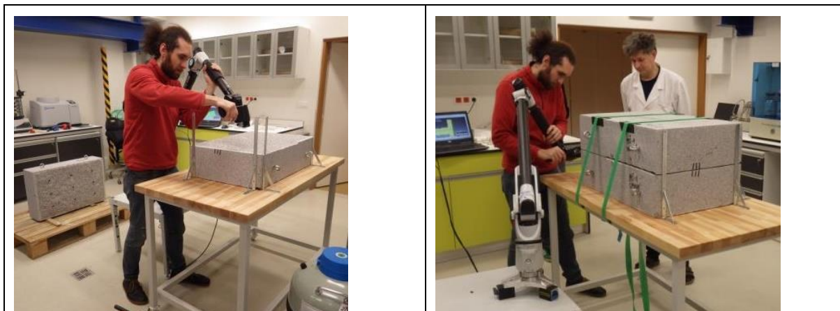
Figure 2-1 3D scanning of fracture surfaces and reassembled block (TACR TH02030543)
