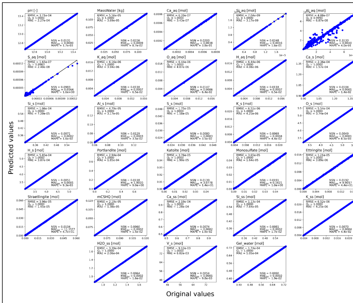
Figure 9 – True (or original) versus DNN-predicted model output values for an independent dataset of a complex cement test case. The “original” values are obtained by running the PHREEQC geochemical solver while the “predicted” values are the computationally way much cheaper DNN predictions.
