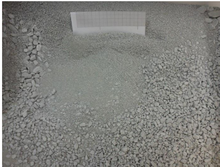
Figure 11: MX-80 bentonite pellets used in the experiment
