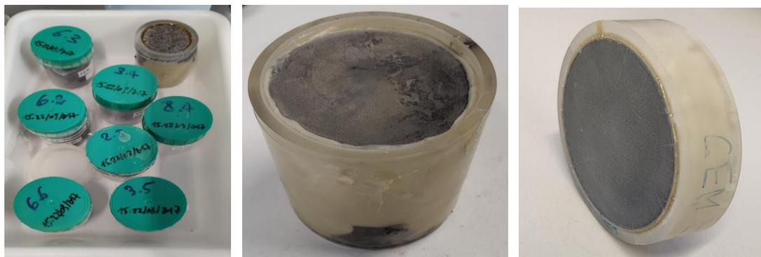
Figure 3-18: Left: Original samples received from [ANDRA]; Middle: the cement sample (5 cm length) that was fitted in a PMMA cylinder; Right: the cut and polished cement sample with 1 cm length.
