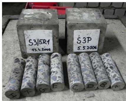
Figure 3-9: Witness samples of structural concrete from the Richard repository
