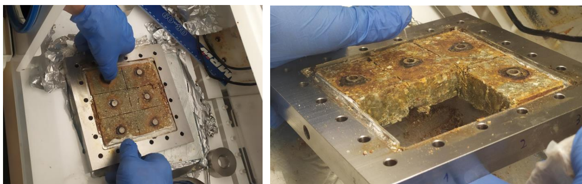
Figure 10 - Pictures of dismantling of FeMo test inside a suboxic chamber. (Left) Sectioning of the sample in six 40 x 60 mm blocks. (Right) Once two of the blocks were extracted, a cross section of the sample can be seen.
