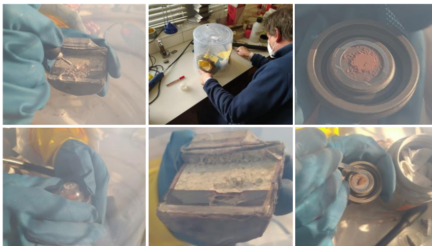
Figure 9 - Preparation of FB-5 interface sample for mineralogical study. The transversal cut shown was performed also under suboxic conditions for the SEM-EDX study.
