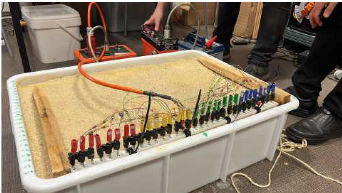
Figure 4-3 – Mock-up scale experiments for verification of IP models. The matrix is made of pure sand. Six samples of bentonite-sand mixtures were buried in the matrix. The acquisition was conducted with 32 electrodes along 19 lines.
