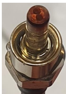
Figure 85: Grafting of NR on the end of a two-way metallized optical fiber.
