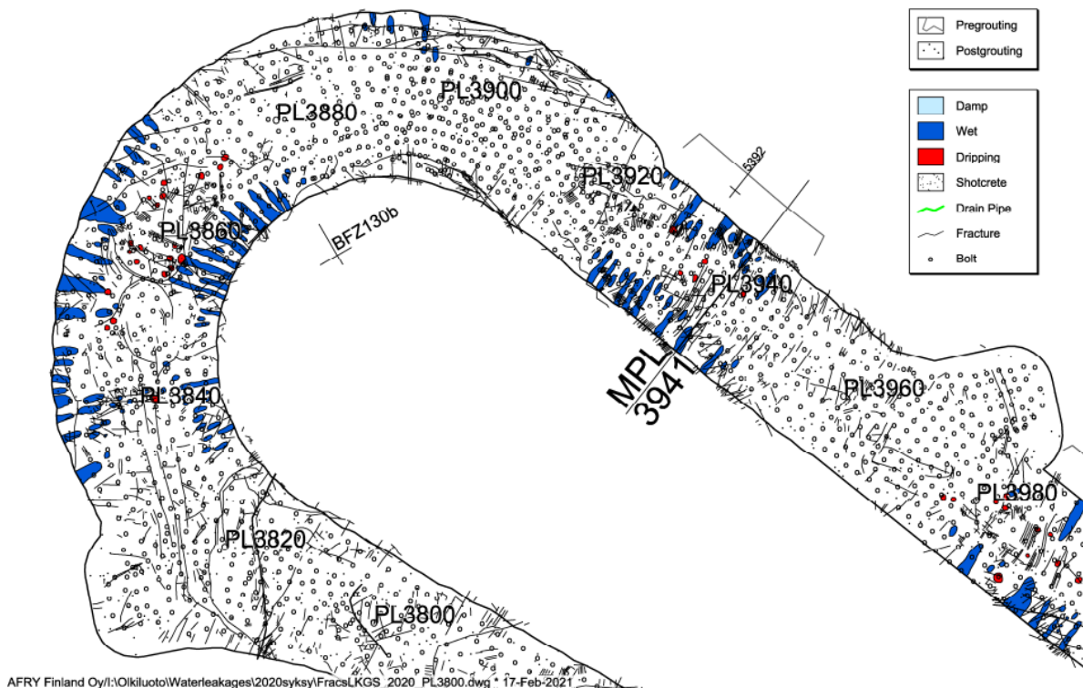
Figure 55: Water logging map of PL3800-PL3980. The map corresponds to images in Figure 53 and Figure 54.
