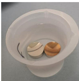
Figure 91: Two stainless steel mirrors, one grafted and the other not grafted.
