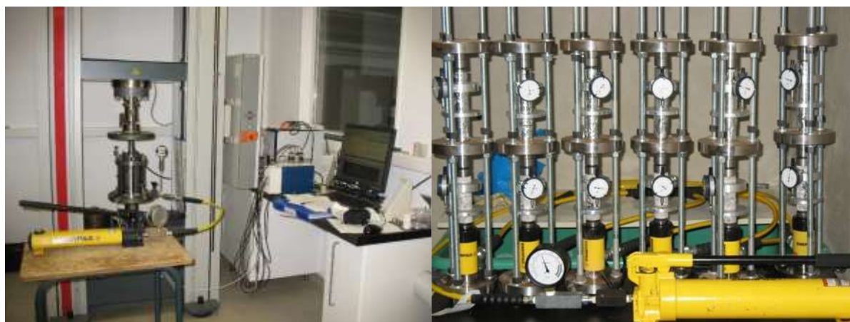
Figure 7-11: Experimental setup for the triaxial (left) and creep tests (right) [16].
