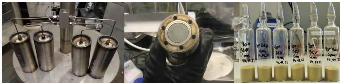
Figure 7: Steel vessels containing steel cells connected by metal capillaries with saturation medium situated in the irradiation area, steel cell with compacted bentonite and glass ampoules with bentonite powder.
