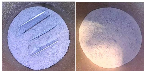
Figure 35: Picture taken with an endoscope camera of the distribution of the carbon steel coupons in the bentonite powder during the initiation of the experiments.
