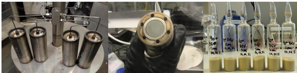
Figure 19: Steel vessels containing steel cells connected by metal capillaries with saturation medium situated in the irradiation area, steel cell with compacted bentonite and glass ampoules with bentonite powder.
