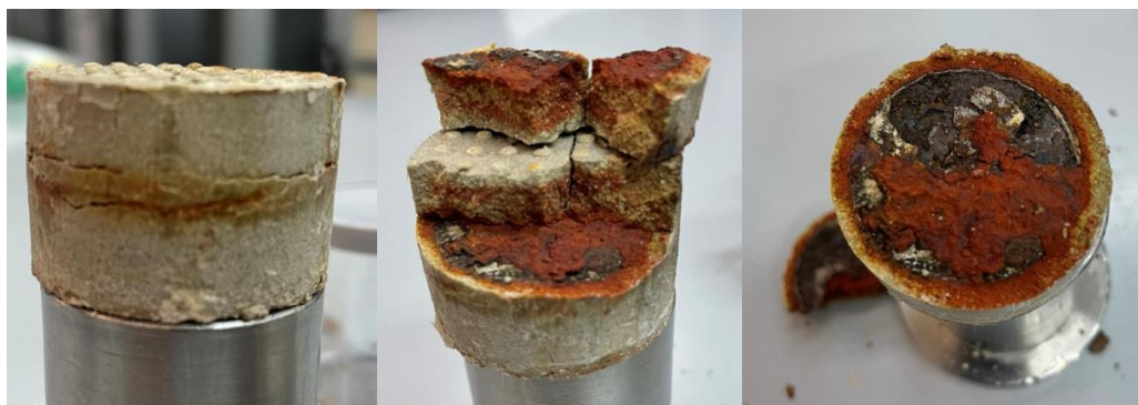
Figure 46. Dismantling of the FEBEX bentonite compacted at 1.4 \text{ g cm}^{-3} with Nagra carbon steel coupon: altered bentonite and corroded carbon steel is shown.
