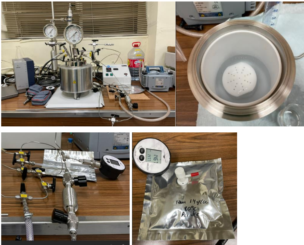
Figure 40. Setup used by CIEMAT for studying coupled redox and thermal transients at 80°C with Nagra-carbon steel / bentonite samples (upper); collection of gas and water samples at the end of the experiment (lower).
