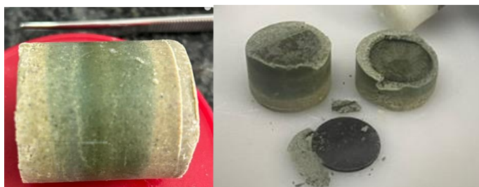
Figure 45. Detail of sampling of FEBEX bentonite at 1.4 \text{ g cm}^{-3} and Nagra carbon steel coupon at the end of the static experiment in the reactor at 80^\circ\text{C} .
