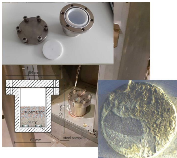
Figure 43. Picture describing the experimental set-up used by GRS for gamma-radiation and thermal transients on SGI/bentonite slurry. Picture at the right-bottom corner shows the optical appearance of the sample after finalisation of the experiment.
