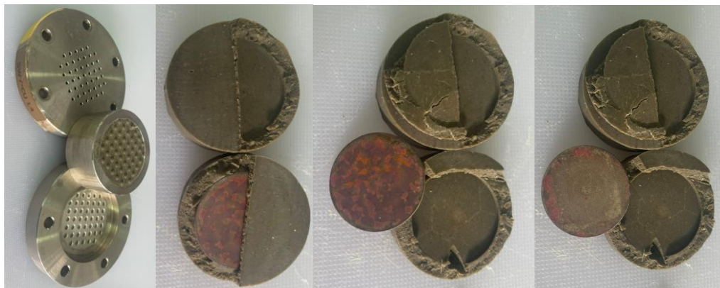
Figure 47. Dismantling the SWy-3 bentonite compacted at 1.4 \text{ g cm}^{-3} with an SKB Cu-OFP coupon.
