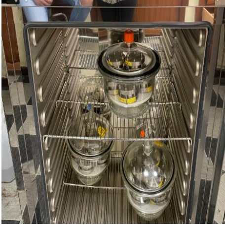
Figure 41. Set-up for convective water vapour thermal flux experiments carried out by CIEMAT under oxic conditions and at 80°C with three bentonites compacted at a dry density of 1.4 and 1.6 g cm -3 with Czech and Nagra carbon steel coupons and Cu-OFP coupons.
