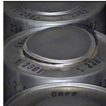
Swelling of bituminous waste
