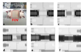
Quantification of water content in the sample by neutron radiography. Sample cell with the neutron field of view (FOV) shown as red square (a); transmission neutron radiographs of an empty cell (b), a dry cement on the left (c), a dry clay on the right (d), a cement-clay interface at time d = 64 days (e) and the same interface at time d = 104 days (f).
