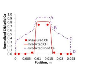
Evolution of Ca in solid phases and portlandite content along depth of sample with w/c ratio of 0.375 and 10% limestone filler after 28 day leaching
