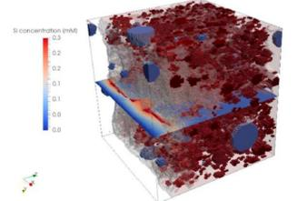
Partially leached microstructure of hardened cement paste. The colours represent different phases of hardened cement paste.
