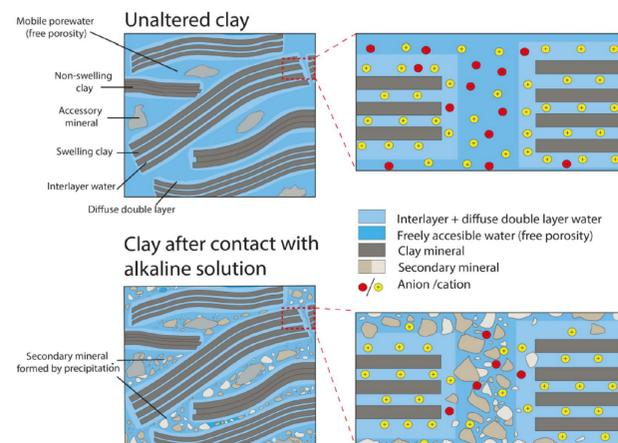
Schematic illustration of clay minerals and respective pore environments for unaltered clay, and for clay after contact with alkaline solution (e.g. cement porewater). Precipitation location (free porosity only or interlayer/diffuse double layer) and precipitation type.
