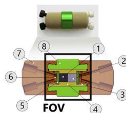
Reaction cell: (1) Cement sample, (2) clay sample, (3) O-rings, (4) PTFE sample holder, (5) PEEK frits, (6) solution reservoirs within PEEK caps, (7) PEEK caps, (8) aluminum holder
