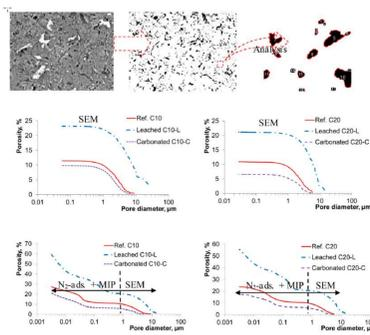
(Top) Segmentation and pore identification from SEM (Middle) Average cumulative porosity derived from SEM (Bottom) Combining N<sub>2</sub>-adsorption, MIP and SEM
