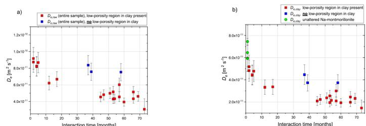
Evolution of the average diffusion coefficient (De) of HTO for (a) the entire system (De,raw) composed of filters, cement and clay); and (b) for the clay part only (De,clay).
