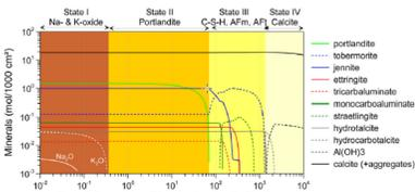
(Top) Cement phase composition during hydration of 100 g of CEM-I OPC clinkers (Bottom) Cement phase evolution during calcium leaching with rain water. Calculations are performed using CEMDATA 18 database, in HPGeochemistry (PHREEQC-version embedded in HPX)
