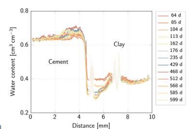
Evolution of profiles of water content with reaction time (in days) across interface. The regions blanked out in the figure are artefacts originating from the joints of the aluminum holder of the cell
