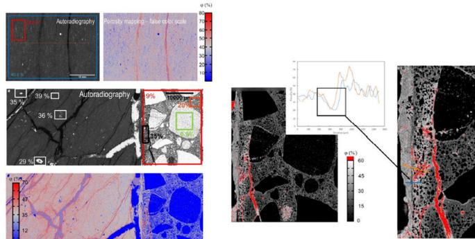
(Left) Porosity maps of Boom Clay obtained by autoradiography (Top) and spatial distribution of porosity at concrete, clay sides and the interface (Middle) and porosity (bottom) mapping of concrete and clay after 14 year interaction at in-situ conditions (Right) Evidence of concrete porosity decrease at clay interface after 14 year interaction with Boom Clay (All measurements by BRGM)
