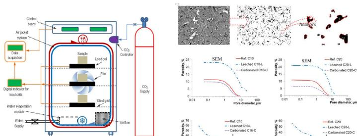
Temperature, relative humidity and CO<sub>2</sub> controlled climate chamber allowing to automatically log experimental variables such as sample mass changes via a digital acquisition system
