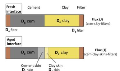
Schematic view of a fresh and aged cement-clay interface sample.
