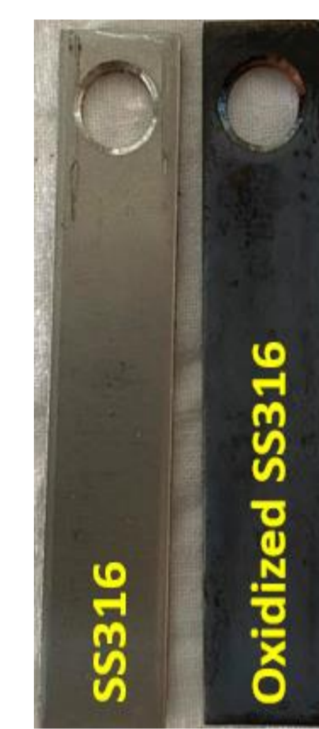
Fig 1. Raw and Surrogate SS 316 sample prepared by SORC
