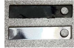
Pristine and oxidized Stainless Steel (316-1.4571)
