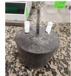
Corrosion tests in mortar under saturated conditions
