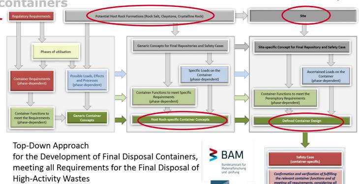
Results of the R&D project KoBrA BMWi funding IDs 02E11527 and 02E11537 relevant loads, effects and processes over
