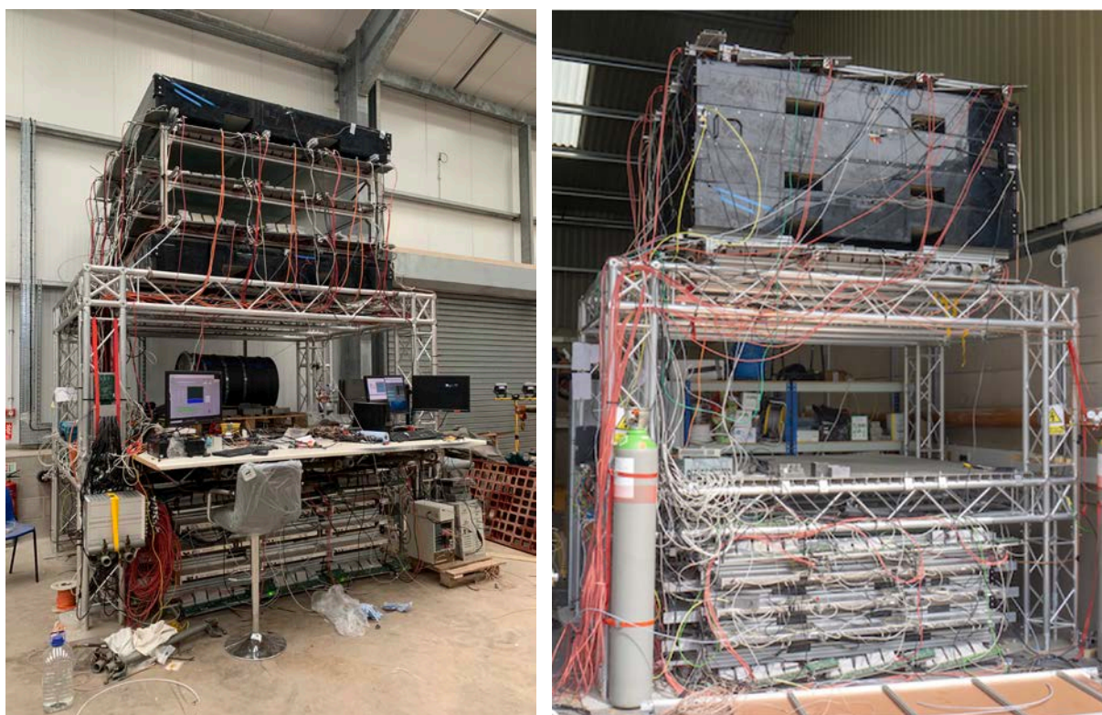
FIGURE 4 - THE CHANCE MUON DETECTOR: THE CONFIGURATION A (RIGHT) AND CONFIGURATION B (LEFT).
