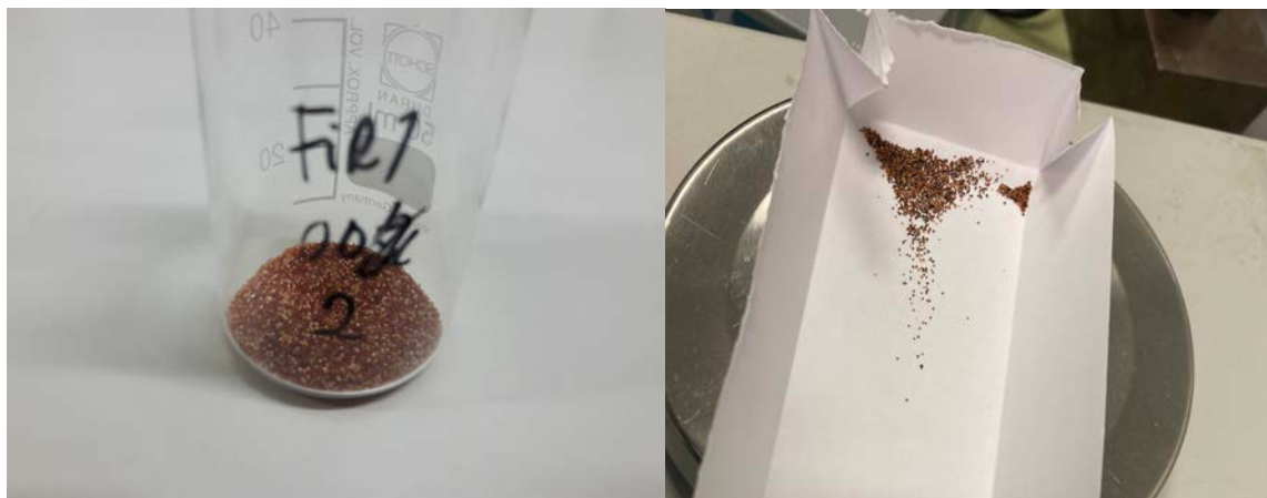
Figure 4. Samples of spent ion-exchange resins used for the measurements. The photo of the resin on the right is taken after partial combustion with the oven and some blackening of the resin can be seen.
