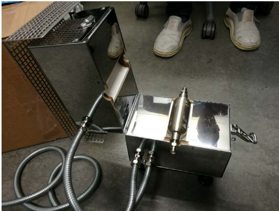
Figure 3 : compact oven designed to enhance the outgassing and for rapid characterisation of the C14 content after full oxidation into carbon dioxide.
