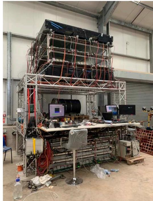
Figure 3.2: The CHANCE detector at Fenswood Farm in the first barn (configuration A) and the second barn (configuration B).
