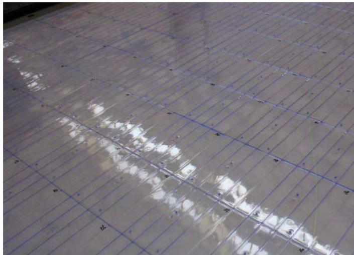
Figure 3.3: Single scintillator trigger paddle consisting of layers of scintillating tiles readout with wavelength shifting fibres.
