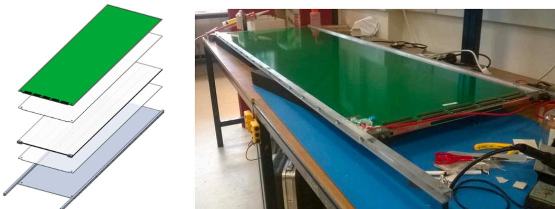
Figure 3.4: Exploded view of an RPC (left) and an assembled RPC (right).
