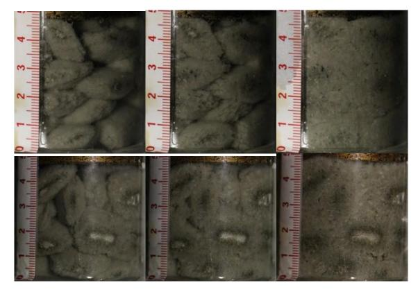
Figure 4-80. Pellet cluster in the acrylic glass tube; pre-tests; after 20, 80 and 320 min
