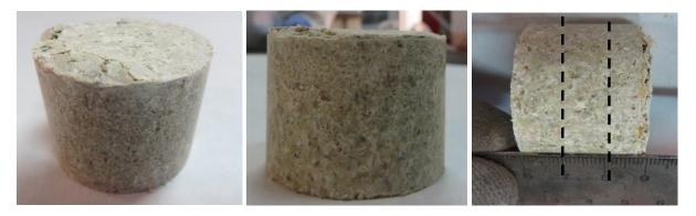
Figure 4-33: Appearance of samples after extraction of the cells and subsampling for postmortem analyses
