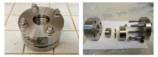
Figure 3-25. Constant volume cells for measurement of retention curves
