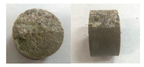
Figure 5-4. Appearance of the cylindrical sample obtained for gas testing in test CW1
