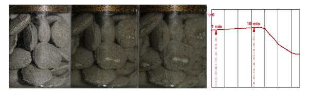
Figure 4-87. Pellet cluster in the pre-test, after 0, 1, and 10 min and swelling pressure
