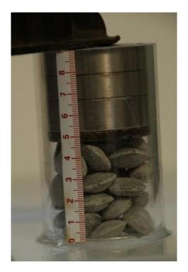
Figure 4-78. Pellet cluster installed in the acrylic glass tube for pre-test 1, dry at t = 0
