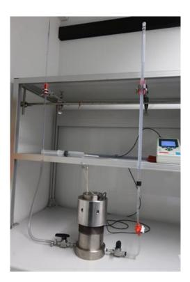
Figure 4-76. Set-up for the test with pellet clusters
