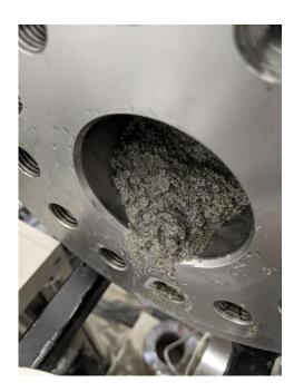
Figure 4-15. During decommisioning of Test 16 (3M NaCI), the clay was found to still be in a fluid state at the end of the vessel which original contained only water. [BGS (C) UKRI]
