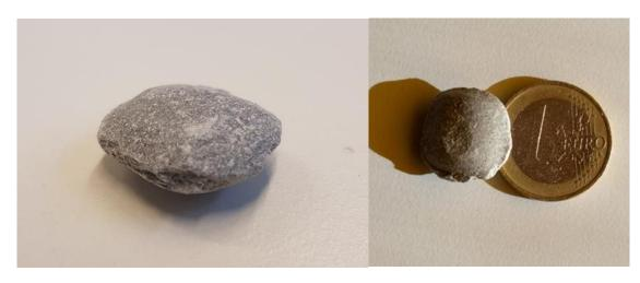
Figure 4-66. MX-80 pellet used in the tests
