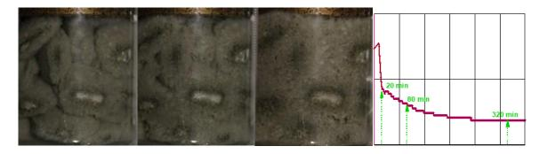
Figure 4-88. Pellet cluster in the pre-test, after 20, 80 and 320 min and swelling pressure
