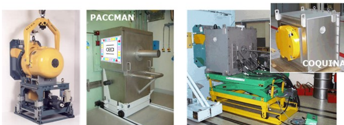
FIGURE 54 PACCMAN, COQUINA, ACTIVE NEUTRON INTERROGATION SYSTEMS PLUGGABLE TO HOT CELLS IN ORDER TO ASSESS URANIUM AND PLUTONIUM IN DIFFICULT TO TRANSPORT HIGH LEVEL WASTES
