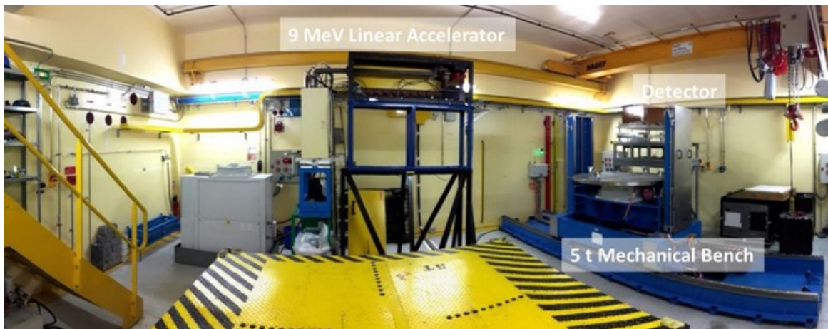
FIGURE 3: THE CINPHONIE BURIED CASEMATE CELL AT CEA, CADARACHE, FRANCE, HOSTING A HIGH-ENERGY PHOTON IMAGING SYSTEM IN THE CHICADE BASIC NUCLEAR FACILITY, WITH A 9 MeV “MINI-LINATRON” LINAC (PÉROT ET AL., 2018)
