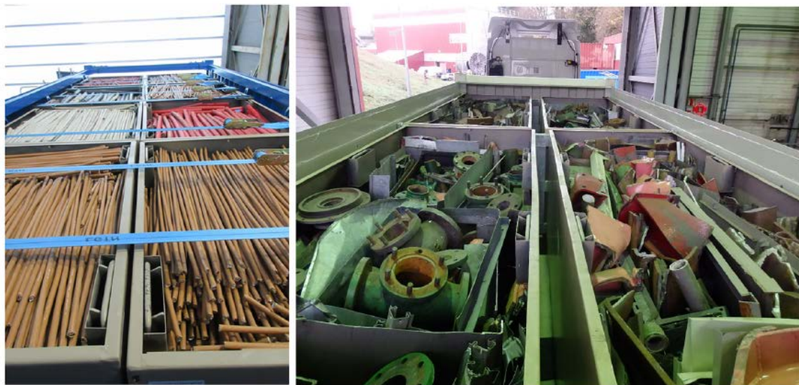
FIGURE 27 : CONTAINER 20 FEET HALF HEIGHT LOADED WITH ACTIVATED CABLES (LEFT) AND ACTIVATED METALLIC (RIGHT) WASTE (FROSIO ET AL. , 2020B)
