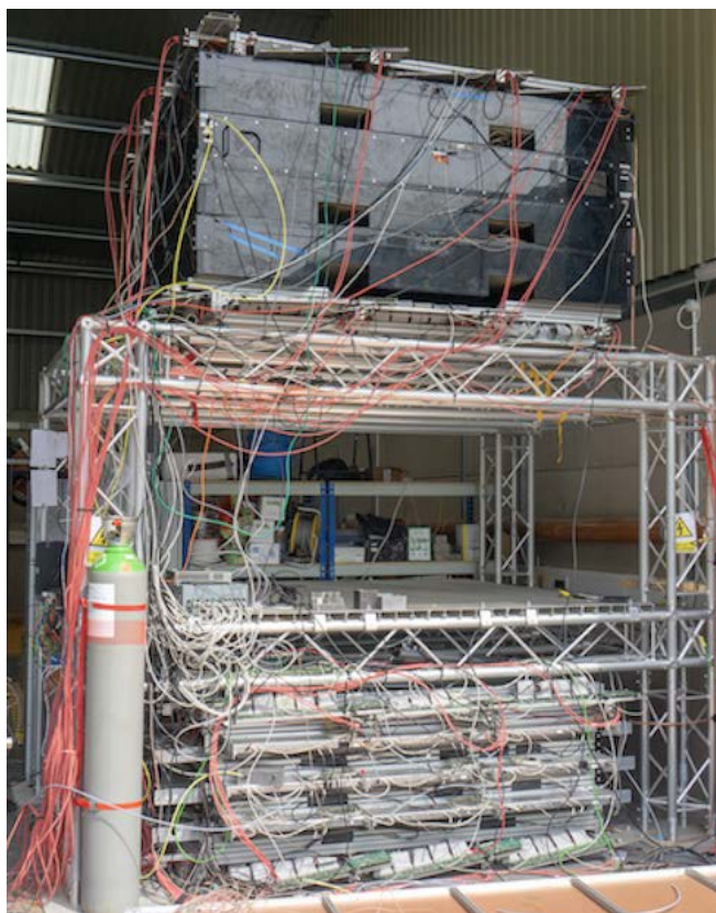
FIGURE 13: THE MUON SCATTERING TOMOGRAPHY DETECTOR SYSTEM OF THE CHANCE PROJECT. SHOWN ARE THE DETECTOR SYSTEMS ABOVE AND BELOW THE EMPTY SAMPLE SPACE CONSISTING OF THREE LAYERS OF DRIFT CHAMBERS AND TWO RPC LAYERS. THE TOP STACK ADDITIONALLY CONTAINS TWO LAYERS OF PLASTIC SCINTILLATORS USED AS TRIGGERS. THE DETECTORS COVER AN AREA OF APPROXIMATELY 1.8 \times 1.8 \text{ m}^2
