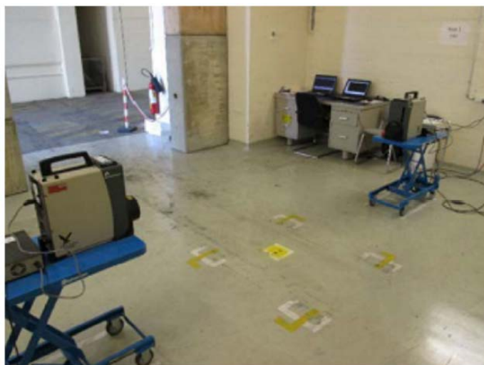
FIGURE 28 : GAMMA SPECTROSCOPY PERFORMED IN A DEDICATED AREA FOR IN-SITU MEASUREMENTS. THE WHITE MARKS ON THE FLOOR REPRESENT THE LOCATION OF THE 1.35 M 3 PACKAGE. TWO HPGE DETECTORS ARE USED TO EVALUATE THE GAMMA EMITTERS RADIONUCLIDES IN THE PACKAGE (FROSIO ET AL. , 2020B)
