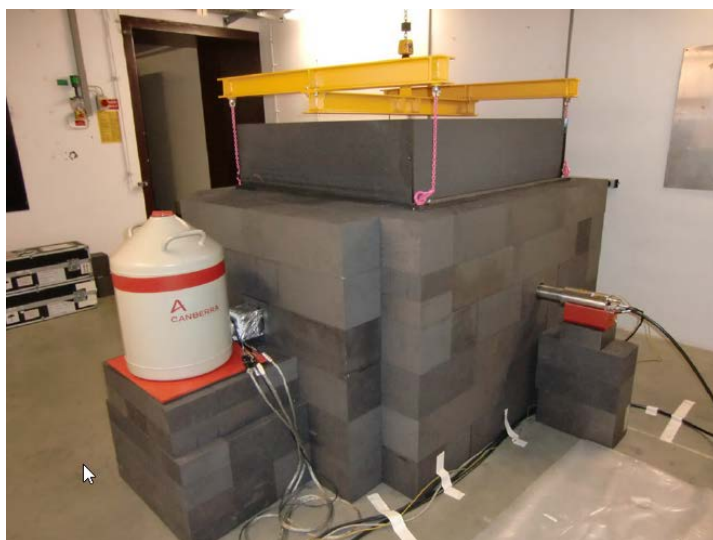
FIGURE 43 : THE FACILITY MEDINA FOR THE ASSAY OF 200-L DRUMS WITH THE HPGE-DETECTOR IN FOREGROUND AND THE 14 MeV NEUTRON GENERATOR ON THE RIGHT (MAUERHOFER AND HAVENITH, 2014)
