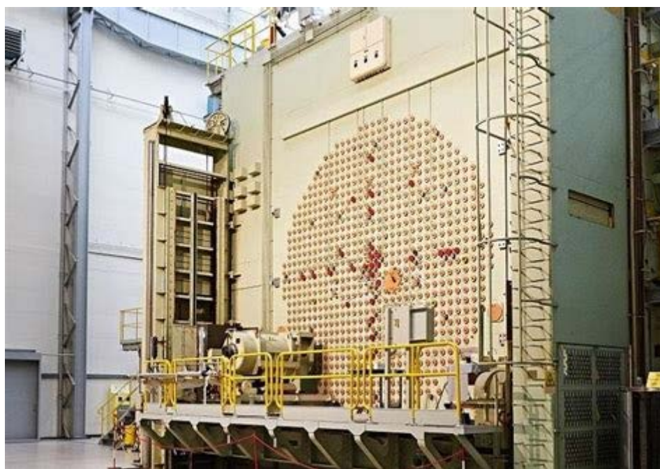
FIGURE 42 : BR1 reactor at SCK CEN, used for neutron activation analysis
