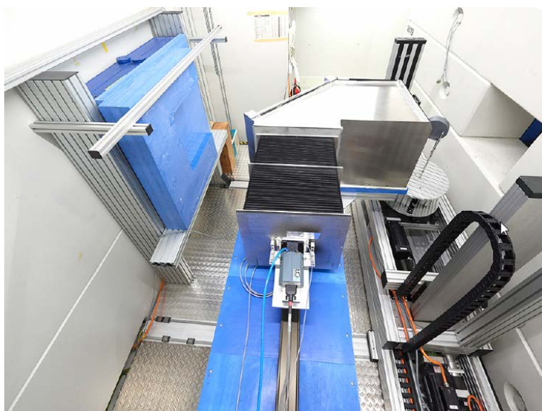
FIGURE 14: INSTRUMENT NECTAR: THE FISSION NEUTRONS ARE COMING FROM THE RIGHT, PENETRATING THE SAMPLE FIXED ON THE MANIPULATOR, AND ARE DETECTED BY A CCD-BASED SYSTEM (CENTER). A BEAMSTOP (LEFT) MINIMIZES SCATTERED RADIATION (BÜCHERL AND SÖLLRADL, 2015)
