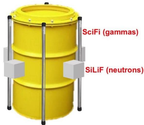
**Figure 6.** A possible arrangement of SciFi and SiLiF detectors around a radwaste package.
