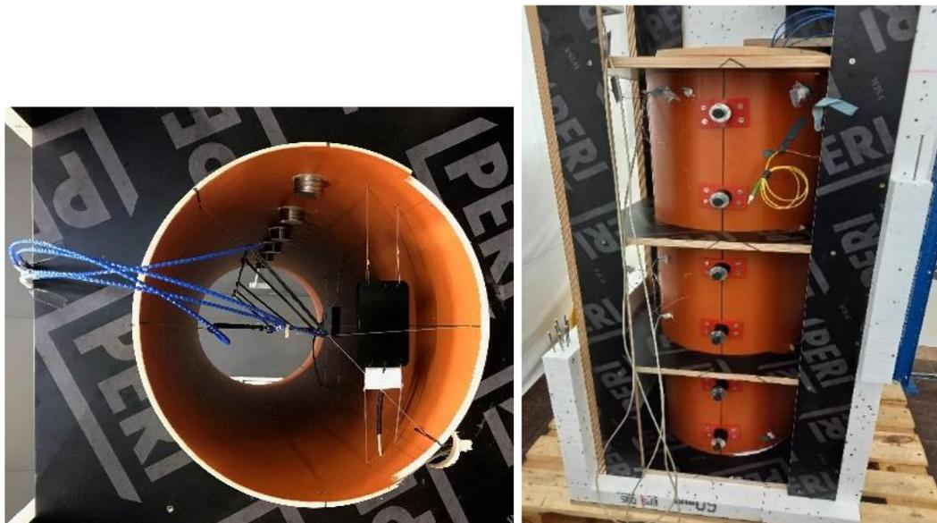
**Figure 10.** Test setup (before concreting) with RFID sensor and cabled sensors for comparison.
