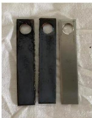
**Figure 7.** Oxidized metallic samples and one unoxidized sample (right) received from SORC.
