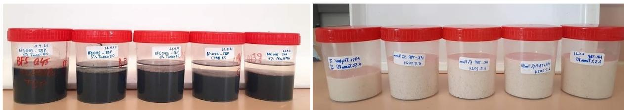
**Figure 6.** State of BFS geopolymer-waste (left) and MK geopolymer-waste (right) with the addition of surfactants after 3 days of mixing.
