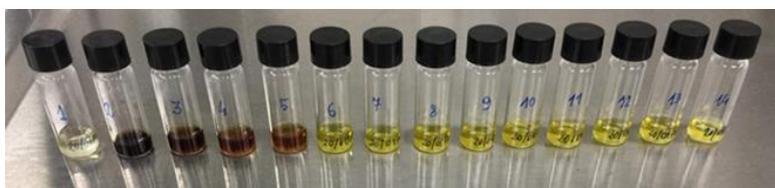
**Figure 6.** Colour shift of resin solution over time for the Fenton-like wet oxidation process
