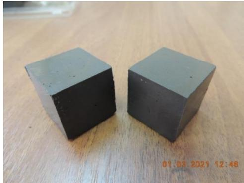
**Figure 8.** Geopolymer samples with 30% of Shellspirax oil.
