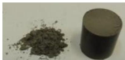
**Figure 3.** Preparation of material for treatment at KIPT: crushed geopolymer-ash material (left), alongside a pressed green body of the same material ready for thermal treatment (right).
