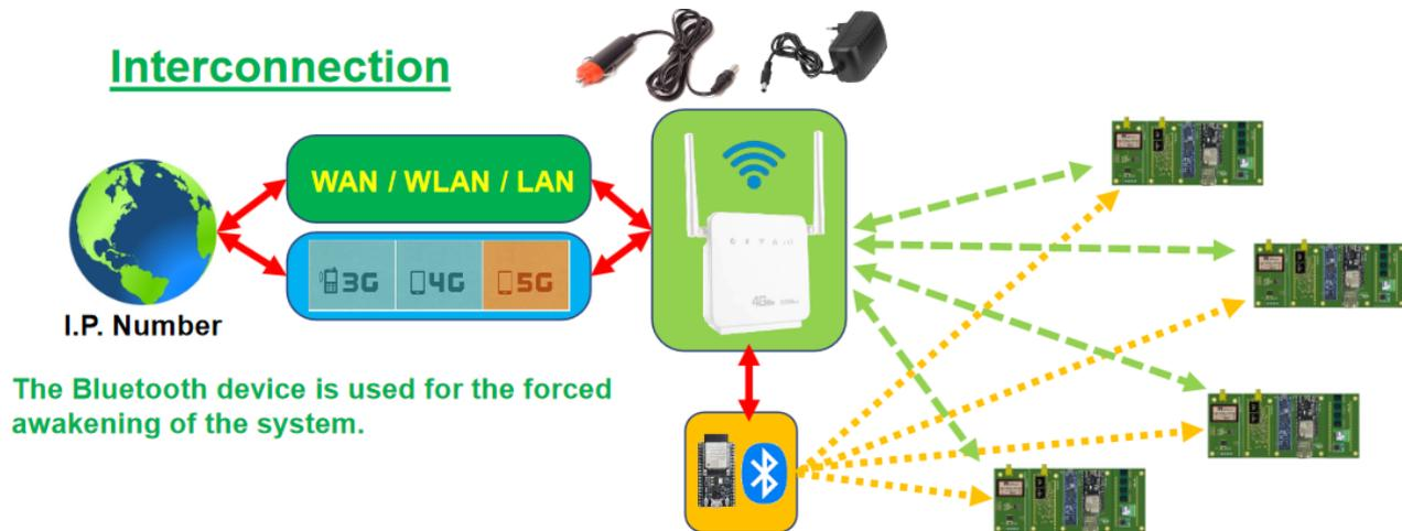
**Figure 8.** Possible interconnection scheme for the detector read-out electronic boards and the external world, making use of a Wi-Fi/Ethernet Router and of a Bluetooth wake-up device.
