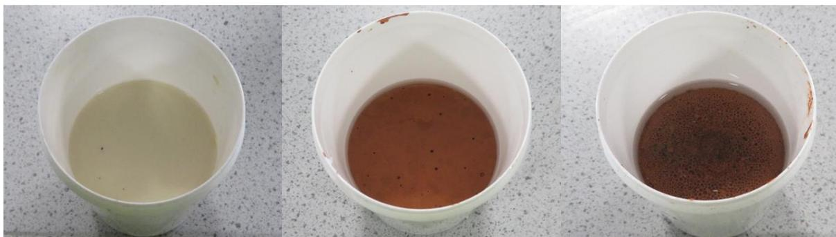
**Figure 3.** 20 vol% loading of TBP in MetaMax geopolymer (left), 10 vol% loading of TBP in Argicem geopolymer (centre) and 20 vol% loading of TBP in Argicem geopolymer (right).
