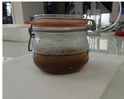
**Figure 10.** Dissolution test of Ni-Fe Oxide powder.
