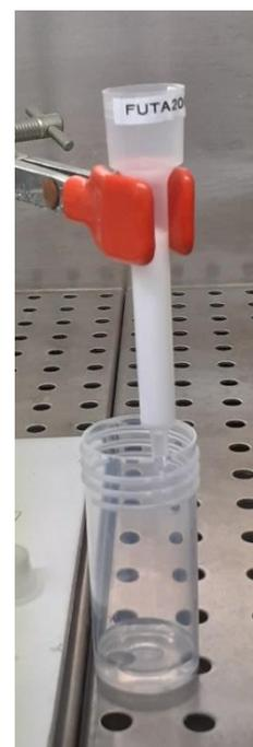
**Figure 4.** Chromatographic resins used for the chemical separation technique intended to apply for the separation of Zr from tetravalent oxides, Mo, Nb and Fe.
