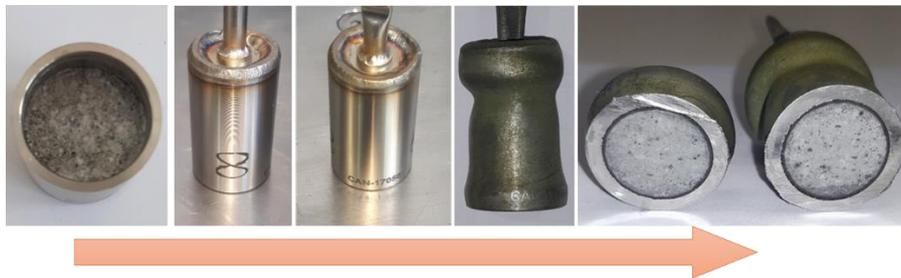
**Figure 2.** HIP treatment of IRIS ashes at USFD from left to right: can packing, welding, crimping, thermal treatment (1250 °C), and sectioning open the can.
