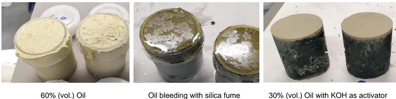
**Figure 1.** Geopolymer formulations with Shellspirax oil.
