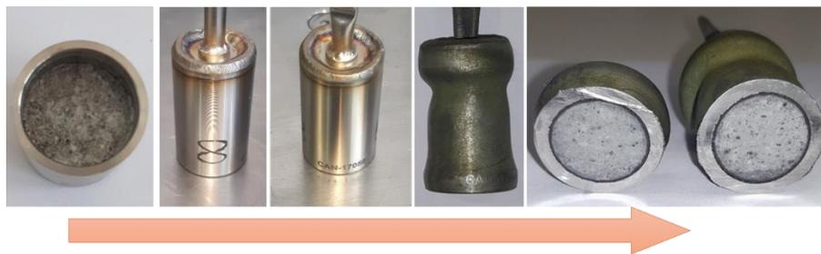
**Figure 2.** HIP treatment of IRIS ashes at USFD from left to right: can packing, welding, crimping, thermal treatment (1250 °C), and sectioning open the can.
