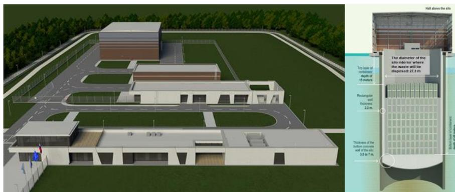
Figure 4: LILW repository facilities and silo cross section
