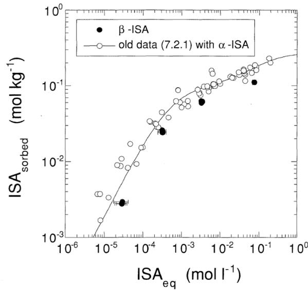
**FIGURE 3-2:** Sorption isotherm of  $\beta$ -ISA on Portland cement at  $\text{pH}=13.3$ . Solid line indicates the modelling of the data obtained for  $\alpha$ -ISA using a two-sites-Langmuir model (Van Loon & Glaus, 1998).
