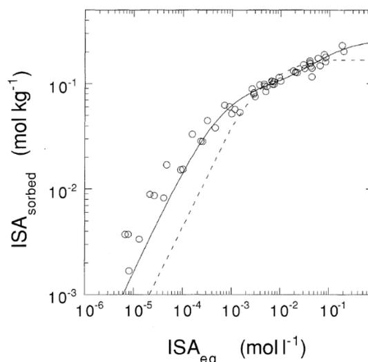
**FIGURE 3-1:** Sorption isotherm of on Portland cement at pH=13.3. Empty circles stand for experimental data, the solid line represents the modelling considering a two-sites-Langmuir model and the dashed line a one-site Langmuir model. (Van Loon & Glaus, 1998).
