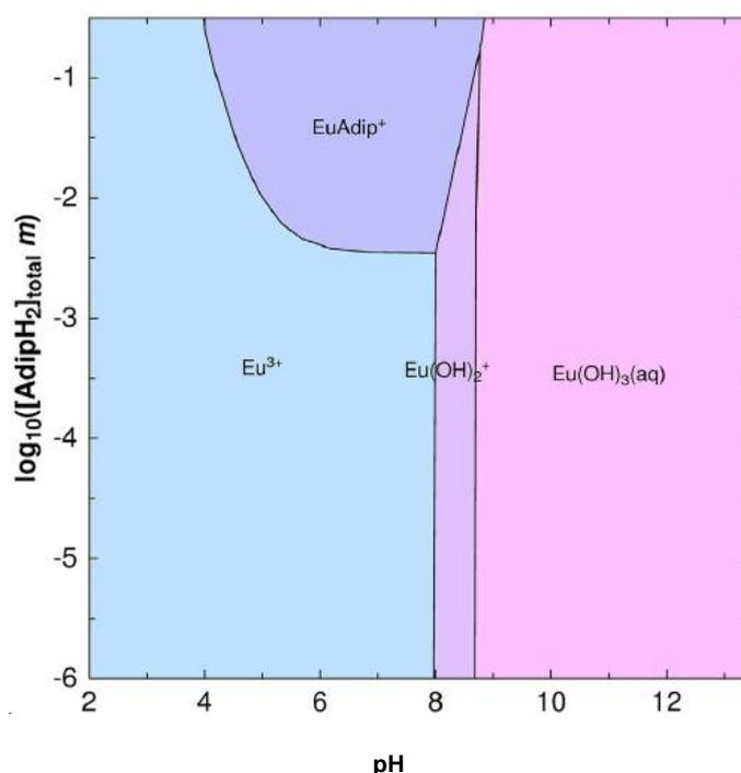
**FIGURE 4-2:** Predominance diagrams of Eu(III)  $10^{-6} \text{ mol} \cdot \text{kg}_w^{-1}$  vs. pH with increasing total adipic acid concentration,  $I=0.1 \text{ mol} \cdot \text{kg}_w^{-1}$  ( $\text{NaClO}_4$ ) at  $P(\text{CO}_2)=10^{-12} \text{ atm}$ . Diagram obtained using Phreeplot software (Kinniburgh and Cooper, 2011) (Fig. 4-2 taken from Fromentin and Reiller, 2018).
