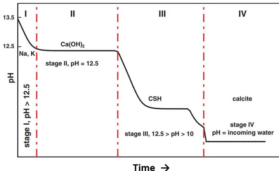
FIGURE 5-6: Schematic diagram illustrating the evolution of pH associated to the gradual degradation of cement-based materials defining four degradation stages (I to IV) (adj. from Ochs *et al.*, 2016).
