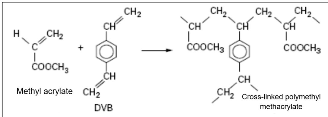
**FIGURE 2-4:** Formation of a polyacrylic skeleton (De Dardel, 1998).
