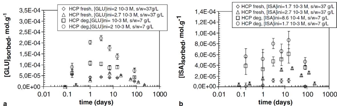
FIGURE 3-4: Evolution of (a) gluconate (GLU) and (b) ISA contents (mol.g<sup>-1</sup>) sorbed on fresh (stage I) and degraded (stage III) cement pastes (Pointeau *et al.*, 2006).
