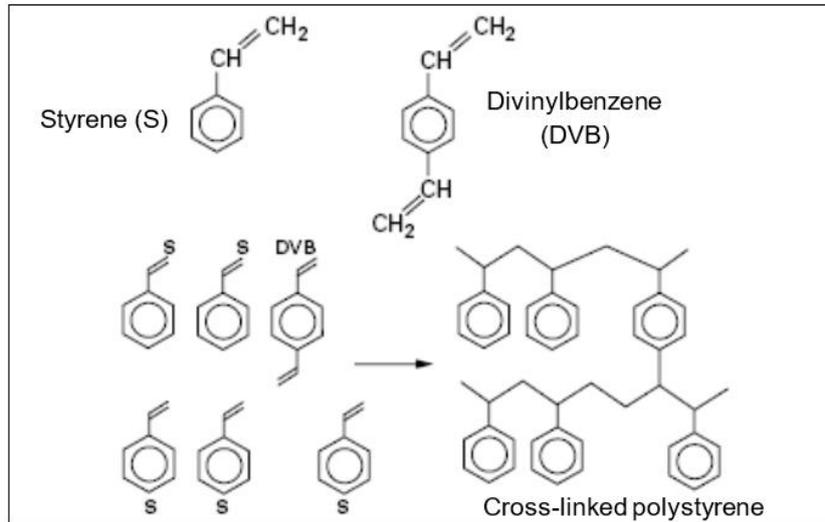
**FIGURE 2-3:** Formation of a polystyrene skeleton (De Dardel, 1998).
