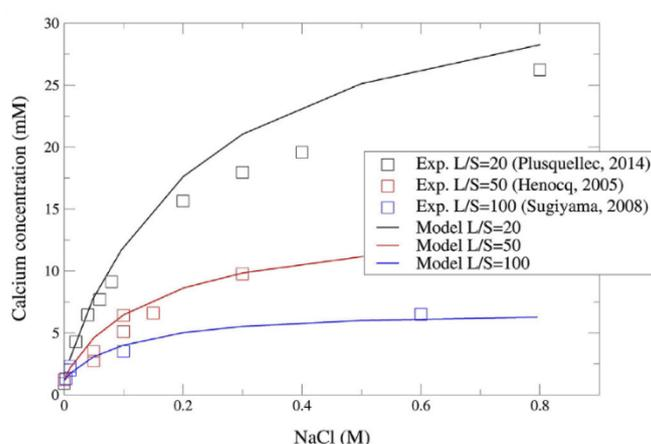
**FIGURE 5-7:** Effect of the Na<sup>+</sup> sorption on the chemistry of C-S-H: evolution of the calcium concentration of C-S-H (C/S=0.8) at equilibrium as a function of NaCl concentration with different liquid-to-solid ratios (L/S). Experiments and modelling (Henocq, 2017).
