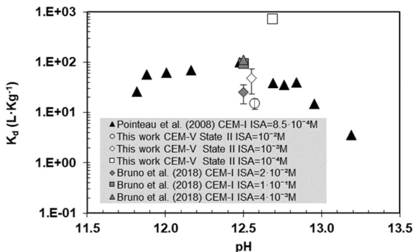
FIGURE 3-5: Comparison of adsorption distribution coefficients ( $K_d$ ) for ISA against pH in fresh and degraded cement pastes. Non-filled symbols are results from Garcia *et al.* (2020) ('this work' in the legend); black filled symbols by Pointeau *et al.* (2008); grey filled symbols by Bruno *et al.* (2018).
