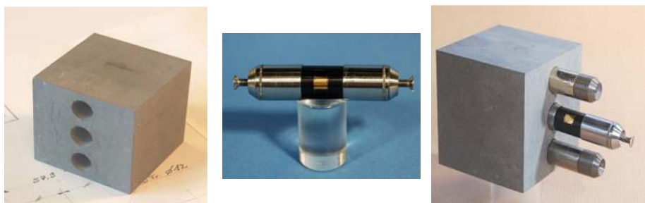
Figure 2-3 – Photographs of the machined brick of argillite, the glass/iron mock-up, and the three specimens inserted in the brick: the glass/iron mock-up studied by Schlegel et al. (2016) in the centre, the gold specimen at the top, and the Armco iron specimen studied by Schlegel et al. (2014) at the bottom.
