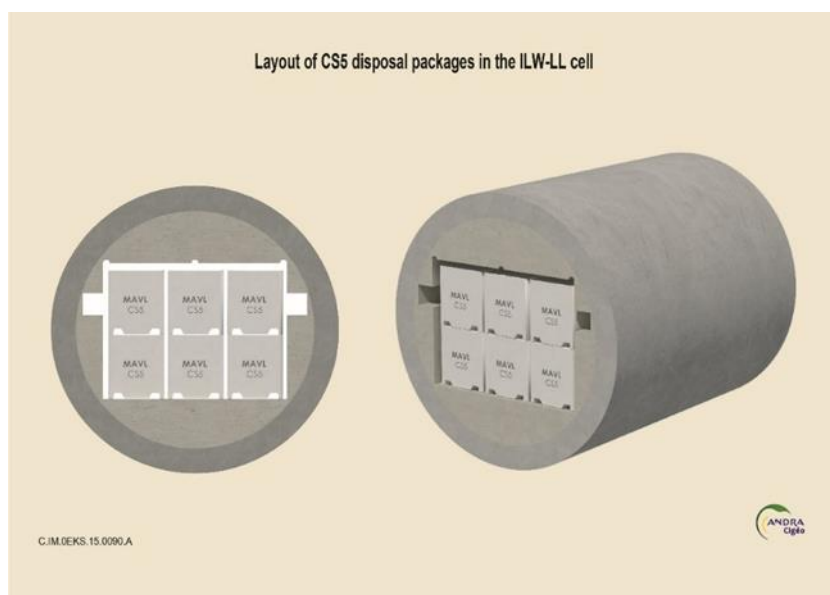
Figure 10-11: Filling of disposal cells with packages type CS5 (at end of basic engineering design).
