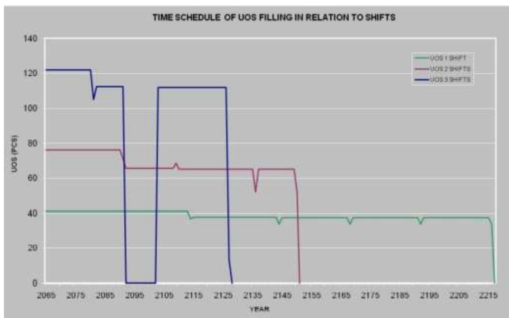
Figure 3.2 - Number of disposed of canisters (UOS) for the one, two and three-shift operation of the repository [32].
