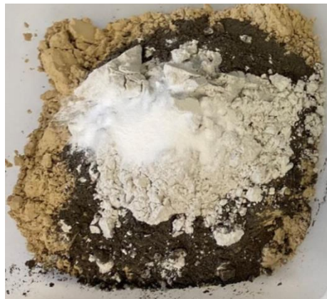
Optimised, tuff-based geopolymer mortar mix with IER ash (POLIMI).
