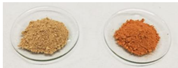
Zeolitized volcanic tuff from Italy for geopolymer matrix formulation (POLIMI).
