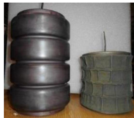
Waste vessel before (left) and after (right) HIP processing, courtesy NNL
