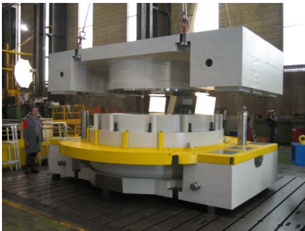
Figure 3: 100 Tonne Mould for Pressing Sand/bentonite Rings
