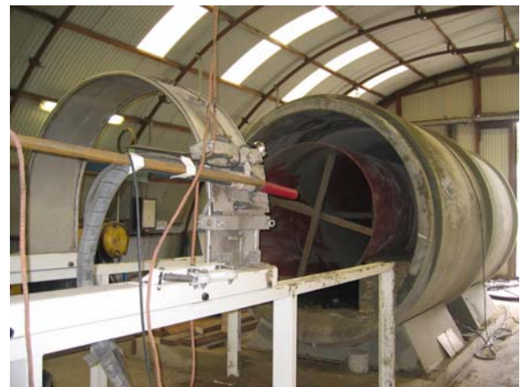
Figure 7: Granular Materials Backfill Test Configuration (June-Oct. 2006)
