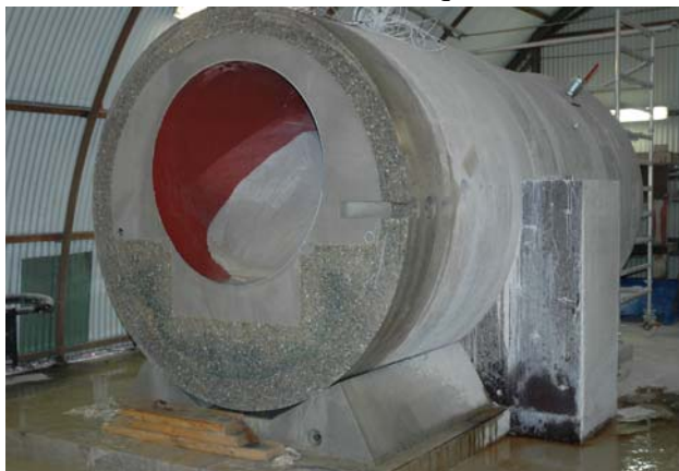
Figure 6: Reduced-scale Mock-up for Grout Backfill Testing, after Slice-cut (Nov. 2006)
