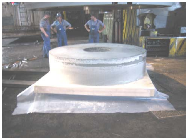
Figure 4: Four Tonne, 2.25m Diameter Sand/bentonite Ring after 45 000 tonnes of Pressure & Stripping from Mould
