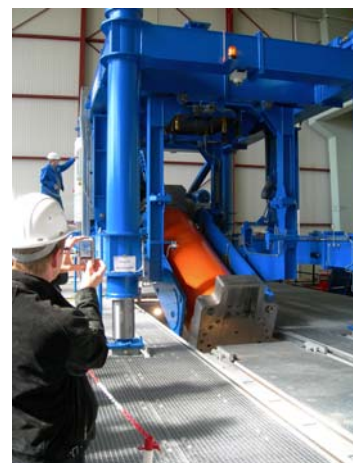
Figure 13: Emplacement Device Manipulating Transfer Cask (Sept.08)
