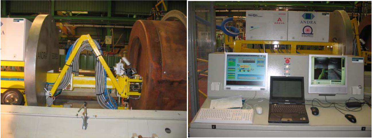
**Figure 21 - Electrical pushing jack connected to the CU1 canister (left) – Control & Monitoring Console (right)**
