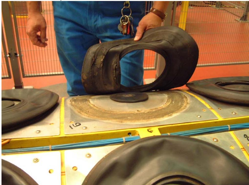
*Figure 24 - Air cushion rubber part separated from support plate*
