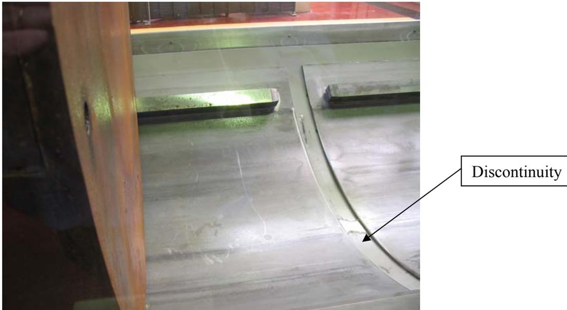
**Figure 23 - Discontinuity between two (2) sections of guiding rails**
